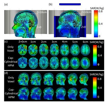
Figure 5. Comparison of SAR in the voxel without and with the application of cap-cylindrical HPM.
