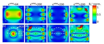
Figure 2. Effect of boundary condition adjustment on  $B_1^+$  mode of the idealized dielectric phantom.
