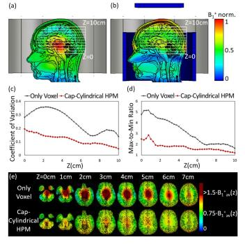
Figure 4.  $B_1^*$  inhomogeneity mitigation by mode-shaping on the voxel using HPMs.
