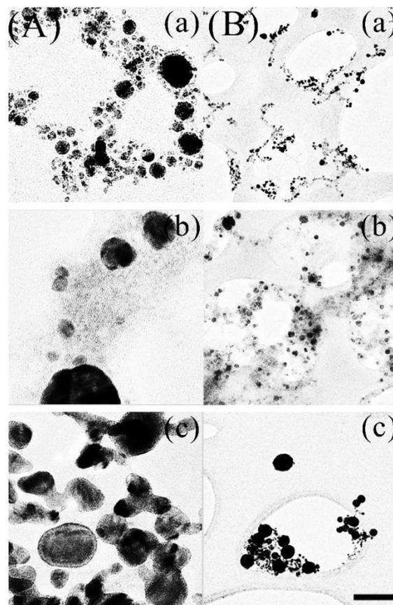
Fig. 6. Transmission electron microscope (TEM) images of (a) Pd, (b) Cu and (c) Ag nanoparticles (NPs), obtained by ablation at the interface of the meniscus of ethanol with the corresponding tilted metal targets, using a 20 J/cm<sup>2</sup> beam fluence. The images in (A) and (B) were taken at different magnifications and the scale bar at the right bottom represents 20 and 200 nm, respectively.
