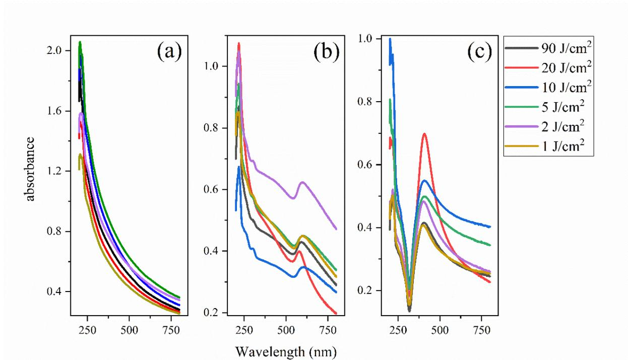
**Figure S3.** Measured UV-Vis absorbance spectra of diluted suspensions of (a) Pd, (b) Cu and (c) Ag NPs in ethanol, shown in different colors, representing the laser fluences that were used for their preparation and given in the upper right corner.
