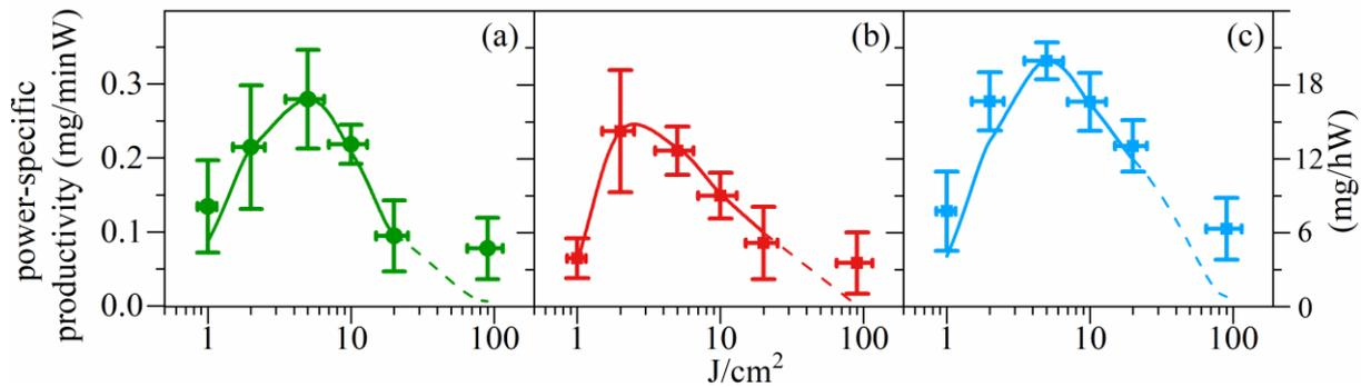
Fig. 3. Measured (scattered) and calculated (lines) power-specific productivities (mg/minW with extrapolation to mg/hW) for (a) palladium, (b) copper and (c) silver as a function of laser beam fluences. The calculated curves were obtained by fitting the productivities in the range of low (solid lines) effective laser fluences,  $F_{eff}$ , for specific simulated plasma absorption coefficients and continued to the high (dashed lines)  $F_{eff}$ .
