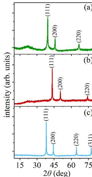
Fig. 8. X-ray diffraction patterns of (a) Pd, (b) Cu and (c) Ag NPs.
