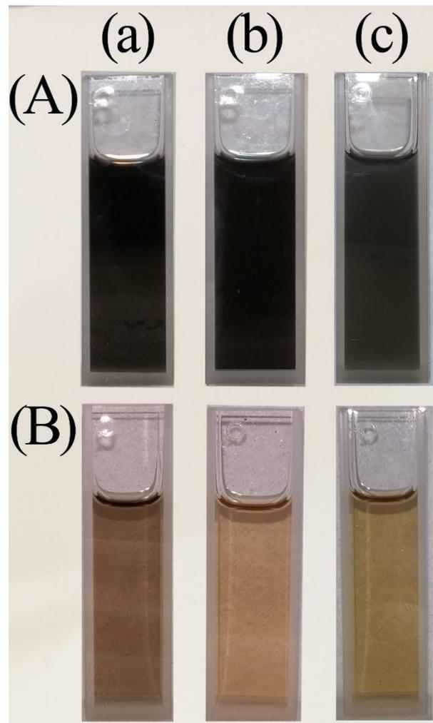
Fig. 2. Ethanol dispersions in cuvettes of (a) Pd, (b) Cu and (c) Ag nanoparticles, obtained following 5 min of ablation. The dispersions exhibit those obtained by ablation at the interface of the meniscus of the corresponding metal targets with ethanol,  $\beta = 2.1 \pm 0.1$  rad, in (A) and those by top ablation of the targets, embedded in 5 ml ethanol ( $\sim 4$  mm height), in (B).
