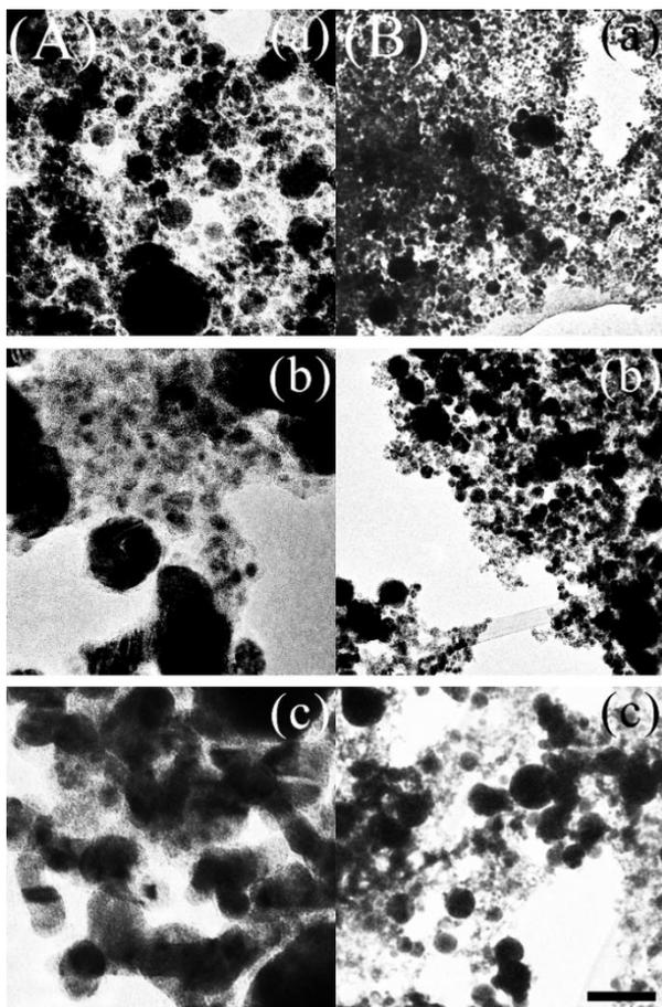
Fig. 7. Transmission electron microscope images of (a) Pd, (b) Cu and (c) Ag nanoparticles, obtained by ablation at the interface of the meniscus of ethanol with the corresponding tilted metal targets, using a  $10 \text{ J/cm}^2$  beam fluence. The images in (A) and (B) were taken at different magnifications and the scale bar at the right bottom represents 20 and 200 nm, respectively.
