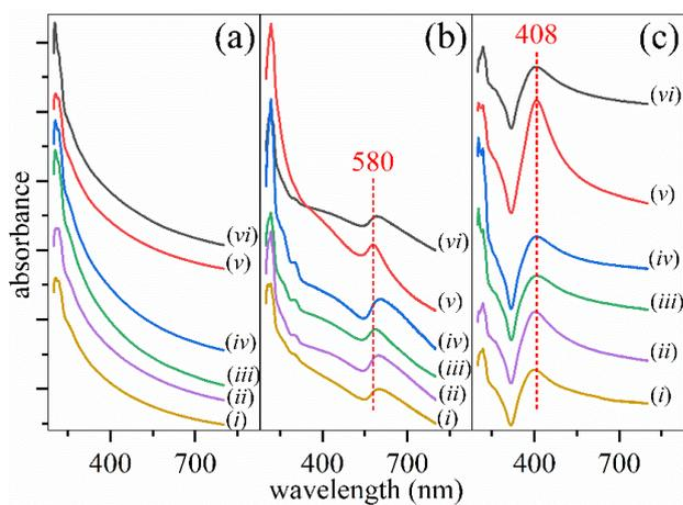
Fig. 5. UV-Vis extinction spectra of (a) Pd, (b) Cu and (c) Ag nanoparticles, ablated from the corresponding tilted metal targets, at the interface with the meniscus of ethanol, using beam fluences of (i) 1, (ii) 2, (iii) 5, (iv) 10, (v) 20 and (vi) 90 J/cm<sup>2</sup>. The wavelengths and the dashed lines mark peak positions of the surface plasmon resonances in (b) and (c). The dashed lines emphasize the relative positions of the peaks in the samples prepared under different fluences.
