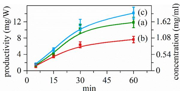
Fig. 4. Measured power-specific productivities (mg/W) and concentrations (mg/ml) for (a) palladium, (b) copper and (c) silver as a function of the time, for the preferable laser fluences of each metal, shown in Fig. 3. The plotted lines are guide to the eyes.
