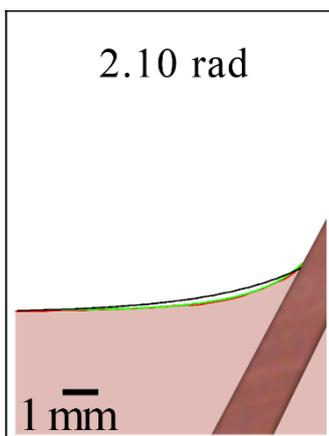
**Fig. S1.** Calculated menisci shapes, marked by lines, in ethanol (red), water (black) and acetone (green) with tilted bulk Cu metal targets at  $\beta = 2.1$  rad (see Fig. 1).
