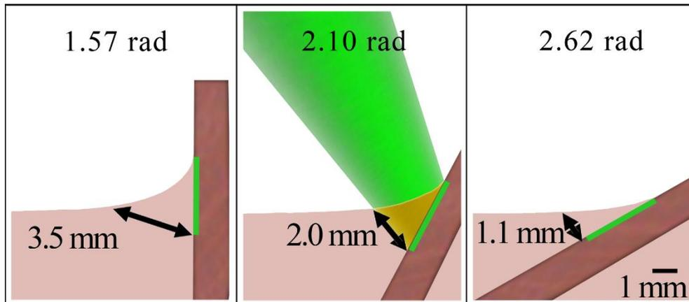
**Fig. S2.** Calculated menisci shapes of ethanol with tilted bulk Cu metal targets, for different  $\beta$  values (see Fig. 1). The beam and the green lines depict the laser spot diameter accessing the target at the lowest used fluence of 0.6 J/cm<sup>2</sup> and the black arrows and the values in mm mark the sampled maximal thicknesses of ethanol above the targets.
