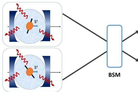
**Figure 4.** Pictorial illustration of the entanglement swapping phenomenon. In each subsystem, the moving qubit is interacting with its own environment. Because of the nonperfect reflecting mirrors of the cavities, the photons can leak out of the cavities. Then a Bell state measurement is performed on these photons establishes the entanglement between the qubits.
