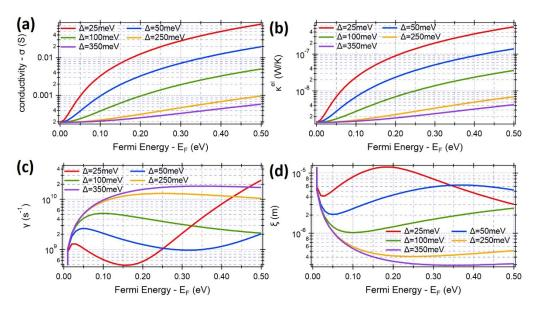
**Fig. 4.** Calculated physical parameters for graphene with different charge neutrality points  $\Delta$ . Calculated conductivity  $\sigma$  (a), electron thermal conductivity  $\kappa^{el}$  (b), cooling rate  $\gamma$  (c), and cooling length  $\xi$  (d) of graphene with  $\sigma_0 = 5(e^2/h)$ , and  $\Delta = 25$ , 50, 100, 250 and 350 meV, respectively. Calculations were performed with electron-phonon coupling strength  $g \approx 0.2294$ .
