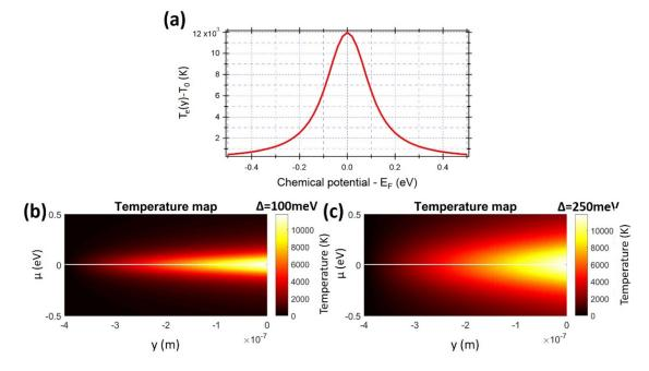
**Fig.6.** (a) Temperature rise in a graphene as a function of the chemical potential and (b), (c) temperature map in a graphene for different  $\Delta$ : (b)  $\Delta$ =100 meV and (c)  $\Delta$ =250 meV.
