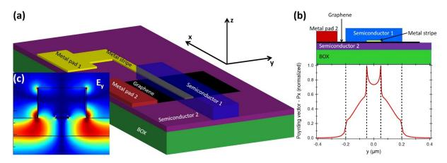
**Fig. 1.** (a) Schematic of the proposed graphene photodetector with a photonic waveguide integrated with the photodetector on the same material platform. Here Semiconductor 1 and Semiconductor 2 are taken as Si. (b) Cross-section through the structure with the Poynting vector  $P_X$  showing a field distribution in a direction of the external electrode (Metal pad 2). (c) In-plane electric field component of the LR-DLSPP mode.
