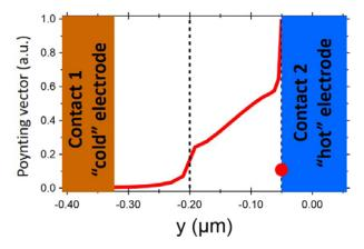
**Fig. 2.** A proposed PTE channel photodetector with the Poynting vector  $P_X$  with the field distribution between metal stripe (Contact 2 - "hot" electrode) and the external electrode (Contact 1 - "cold" electrode).
