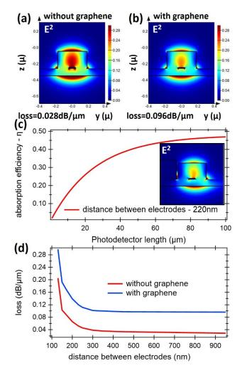
**Fig. 3.** (a), (b) Calculated  $E^2$  of the LR-DLSPP waveguide mode with corresponding losses for structure without graphene (a) and with graphene (b). (c) Calculated absorption efficiency versus photodetector length for a photodetector with 220 nm separation distance between electrodes. (d) Propagation losses versus distance between electrodes for structures without graphene and with graphene.
