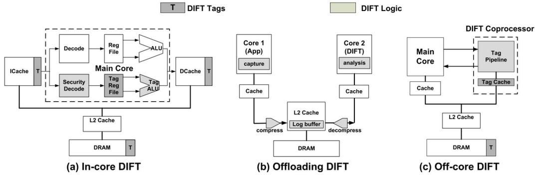
Figure. 1. The three design alternatives for DIFT architectures [5]
