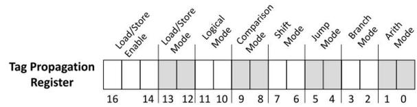
Figure 2. Tag Propagation Register (TPR) proposed in [3]
