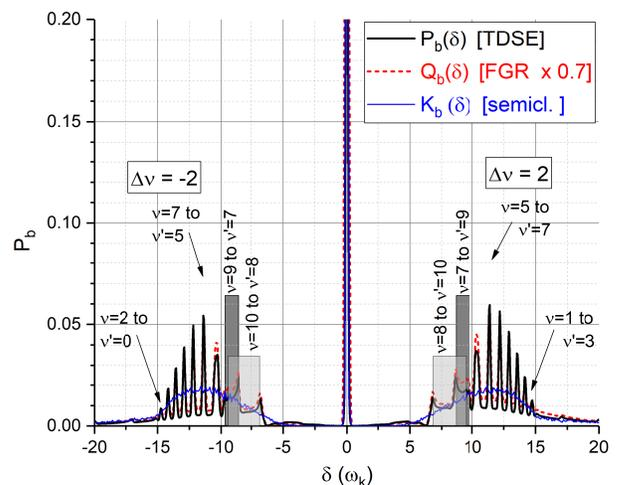
FIG. 4. (Color online) POL modulation spectra  $P_b$  (TDSE),  $Q_b$  (FGR) and  $K_b$  (semi-classical) for  $V_1 = V_2 = 2\pi \times 250$  kHz,  $\tau_{\text{FWHM}} = 400\mu\text{s}$ , and  $T = 10 \mu\text{K}$ .
