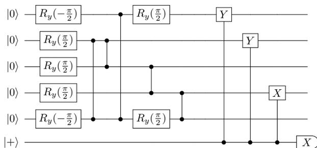
FIG. 6. A noise-robust circuit to encode a logical minus state  $|-\rangle_L$  with the five qubit code. In addition to the first part of the circuit (Fig. 4(a)) which prepares  $|-\rangle_L$ , three two-qubit gates are applied from the ancilla qubit, which is then measured in the  $\{+, -\}$  basis. If measured to be  $-$ , the output is abandoned and re-prepared until the measurement result is  $+$ .
