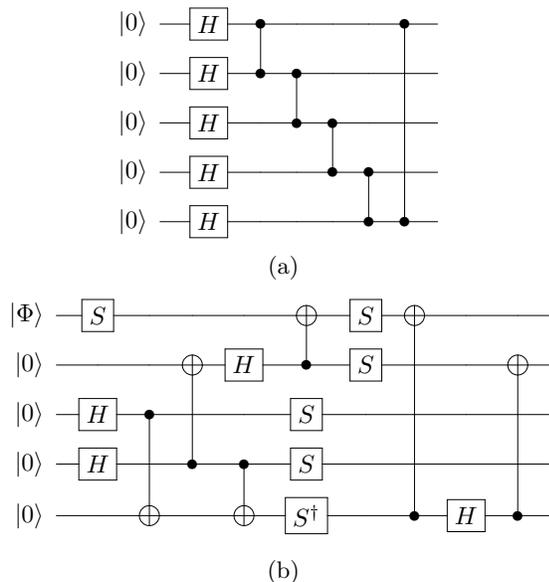
FIG. 1. Encoding circuit for the five qubit code. (a) Circuit to encode the logical minus state  $|-\rangle_L$  [47]. (b) Circuit to encode an arbitrary logical state [14].
