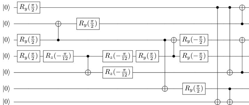
FIG. 5. Circuit to encode a logical magic state  $|T\rangle_L = \frac{\sqrt{2}}{2}(|0\rangle_L + e^{\frac{\pi}{4}i}|1\rangle_L)$  with the seven qubit code. Minimally 9 two-qubit gates are required to prepare the state.
