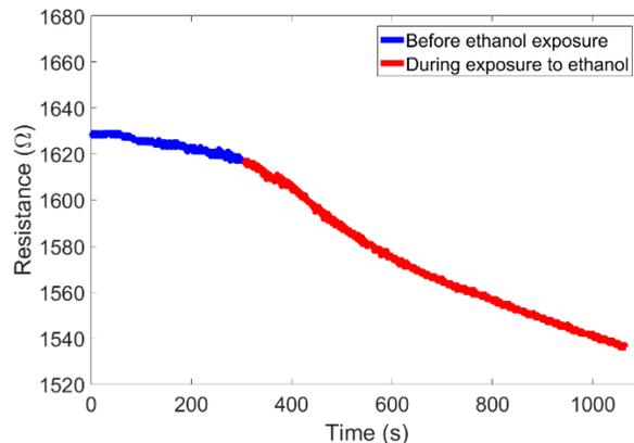
Fig. 5. Resistance ( $\Omega$ ) of the sensor over time (s) in the presence of ethanol, as recorded by the apparatus.
