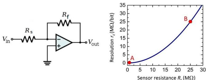
Fig. 3 (a) Diagram of an inverting operational amplifier. (b) Graphical representation of the resolution of our circuit as a function of the sensor resistance (based on (2)). For our circuit, the accessible range is contained between the points “A” and “B”.
