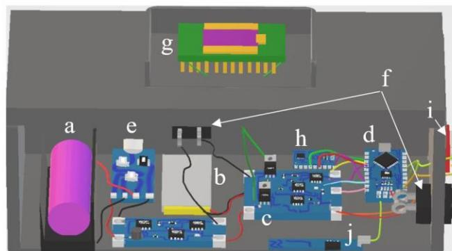
Fig. 1. Design and representation of the portable and wireless signal transducer. The system is composed of: (a) the Lithium ion battery, (b) the lithium polymer battery, (c) the main circuitry of the apparatus, (d) the microcontroller module, (e) the module with a female micro-usb port, (f) the switches, (g) the graphene sensing surface, (h) the ADC, (i) the temperature and humidity sensor, (j) the bluetooth module.
