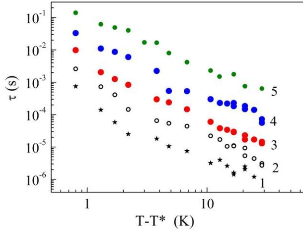
Fig. 2. Temperature dependence of the partial relaxation times  $\tau_i$ ;  $i=1-5$ . The processes are marked with numbers. The main processes 3 and 4 are highlighted with large dots.
