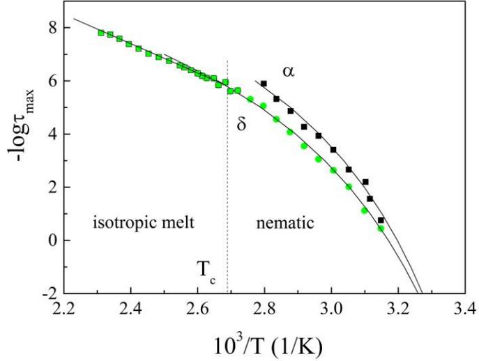
Fig. 4. Dependences of  $-\log \tau_{\max}$  on the inverse temperature for  $\alpha$  и  $\delta$  processes in the isotropic and LC phases of Cop-9.7.
