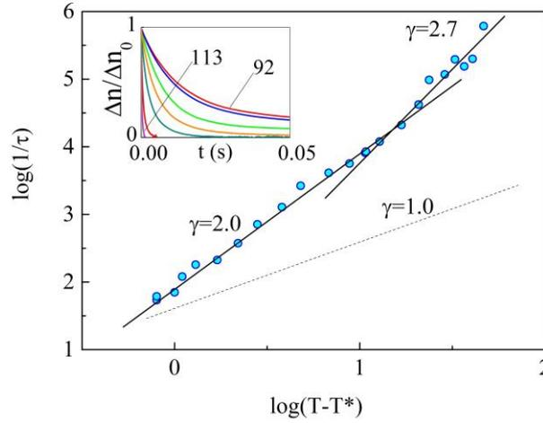
Fig. 1. Temperature dependence of the inverse integral relaxation time  $\tau$  of the orientational order in the isotropic melt of Cop-9.7 polymer. The dashed line corresponds to the theoretical value  $\gamma=1$ . The inset shows the decay curves of the reduced birefringence in the temperature range from 113 to 92 °C.
