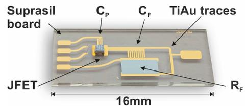
**Figure 1.** Image of a prototype LMFE device for LEGEND-200.
