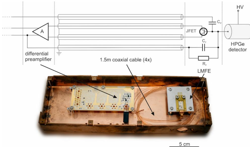
**Figure 2.** Simplified circuit diagram of the LEGEND-200 signal readout electronics (top) and image of a realised prototype of the electronics used in bench-top measurements (bottom).
