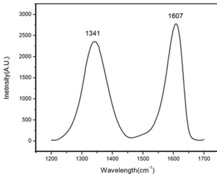
Figure 10. The Raman spectrum of as prepared GO.
