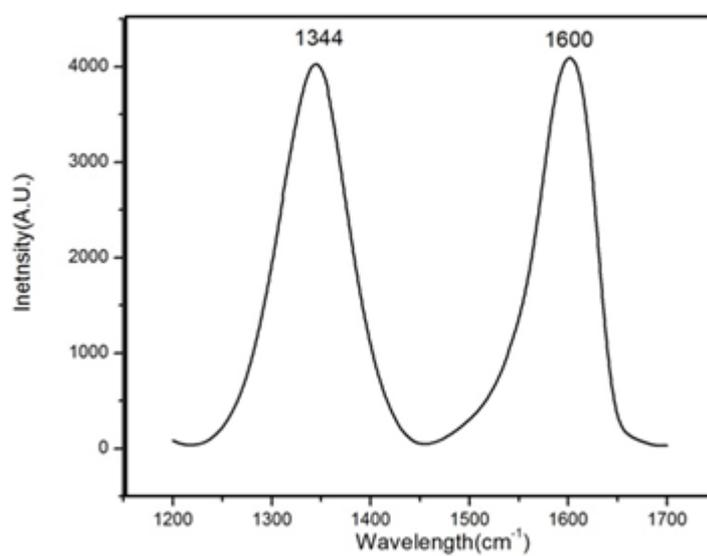
Figure 12. The Raman spectrum of ammonia plasma (5 min at Room Temperature) treated GO.
