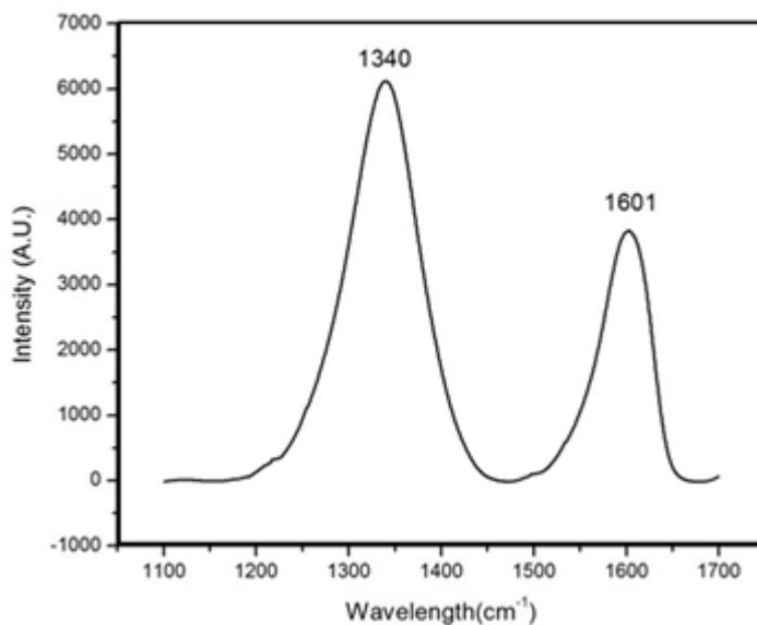
Figure 11. The Raman spectrum of hydrogen plasma (30 sec at 50<sup>o</sup>C) treated GO.
