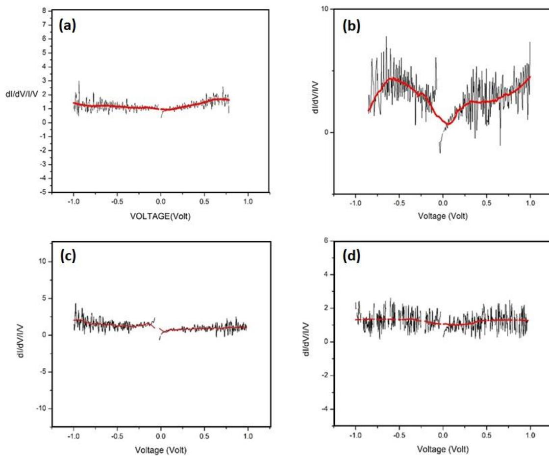
**Figure 6.** The normalized differential tunneling current against bias voltage for (a) ammonia plasma treated GO, transferred onto the Si, (b) for hydrogen plasma treated GO, transferred onto the Si, (c) hydrazine treated GO, transferred onto the Si & (d) for Graphite reduced GO, transferred onto the Si.
