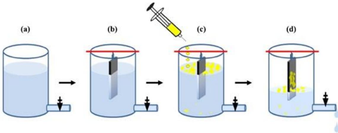
**Figure 3. Successive stages of transfer of GO monolayer sheets by MLB technique: (a) milli-Q water as the subphase in a reservoir, (b) substrate inserted in the subphase, (c) GO solution is spread and (d) transfer of GO sheets by draining of the subphase [20].**
