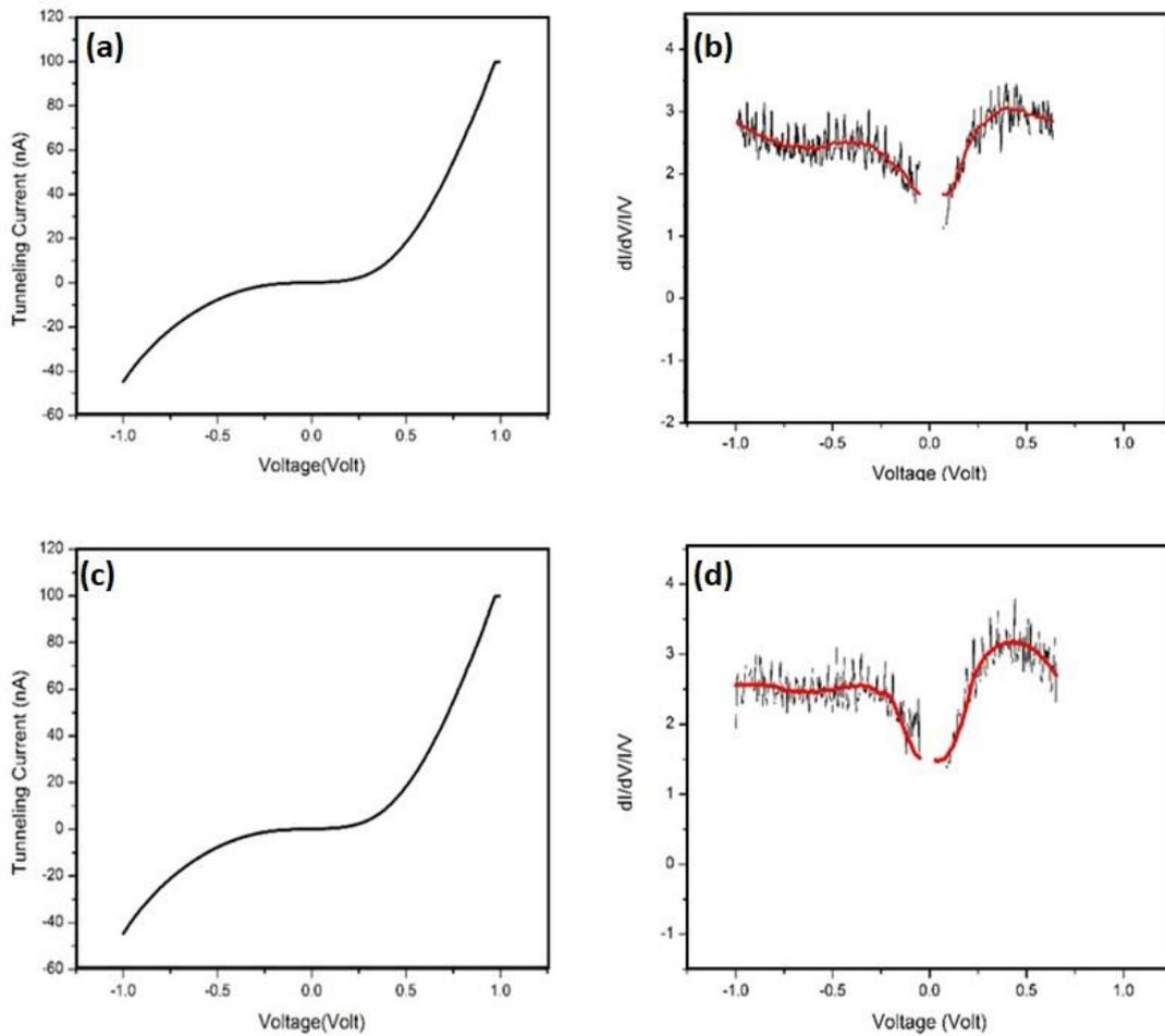
**Figure 5.** The tunneling current against bias voltage for two different GO samples (a) & (c) and the normalized differential tunneling current against bias voltage (b) & (d) for the GO, deposited on Si.
