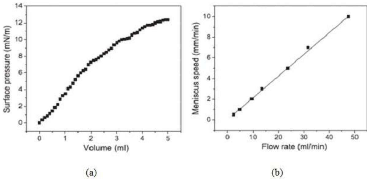
Figure 7. The plots of (a) surface pressure vs volume and (b) meniscus speed vs flow rate, of the spreading GO solution.
