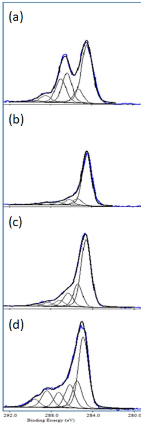
Figure 9. The de-convoluted C-1s spectra of and (a) GO (b) Hydrazine treated GO. (c) 30 sec hydrogen plasma treated GO with 15 watt power at 50°C and (d) 5 min ammonia plasma treated GO with 10 watt power at room temperature.
