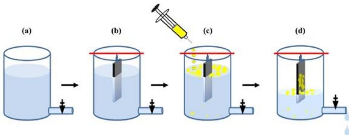
**Figure 3. Successive stages of transfer of GO monolayer sheets by MLB technique: (a) milli-Q water as the subphase in a reservoir, (b) substrate inserted in the subphase, (c) GO solution is spread and (d) transfer of GO sheets by draining of the subphase.**
