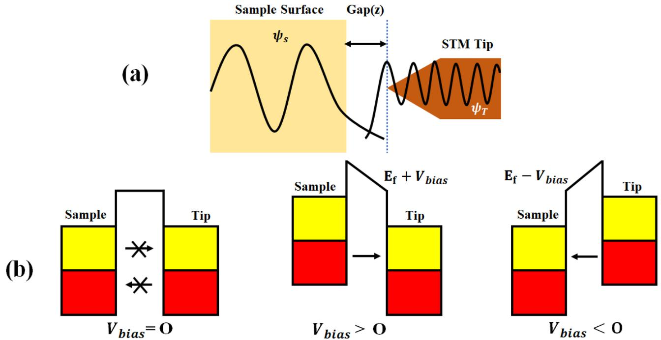
**Figure 1.** (a) Schematic of STM one dimensional tunnelling configuration, (b) Schematic of a metal-insulator-metal tunneling junction. The grey area represents electron filled states and the white area is empty states
