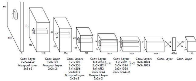
Fig. 2. YOLO Architecture, proposed by Redmon et al [14]
