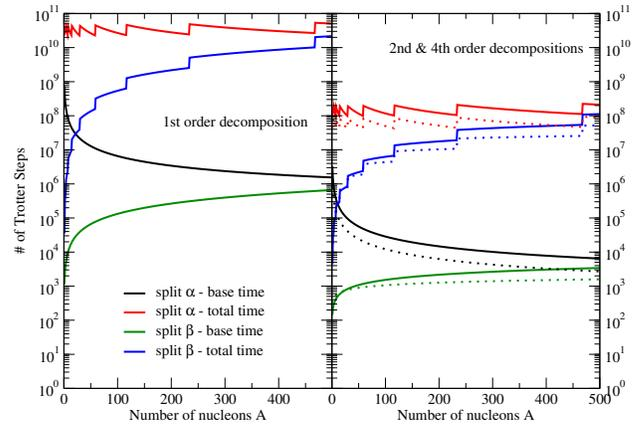
FIG. 1. Estimated number of Trotter steps for both splittings of the Hamiltonian and target resolutions  $\delta\omega = 10$  MeV for Trotter-Suzuki formulae of different order. The left panel shows the linear formulae Eq. (13) and Eq. (14), the right panel shows results for both a second order formula (solid lines) and a fourth order one (dotted lines).
