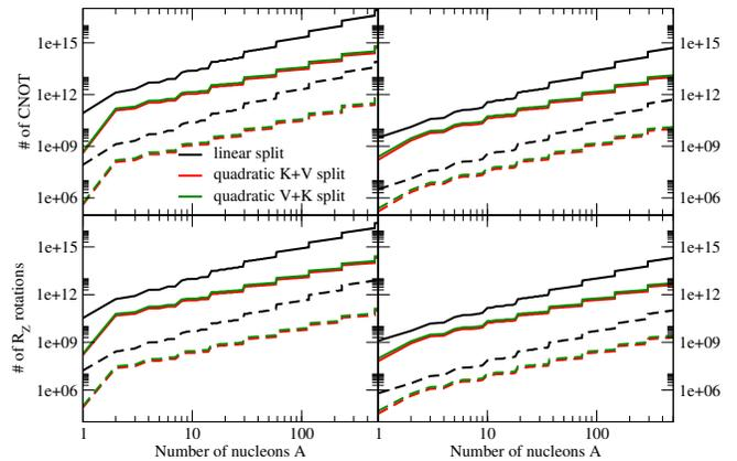
FIG. 3. Estimated gate count, in the CNOT+ $R_z$  basis, of the phase estimation kernel of the linear response algorithm of [17] as a function of nucleon number. Shown are results for the  $\beta$  splitting and both first and second order Trotter decompositions. The left panel is for an energy resolution  $\Delta\omega = 10$  MeV and the right for  $\Delta\omega = 100$  MeV. The solid lines correspond to the serial execution while parallelism is exploited for the dashed ones.
