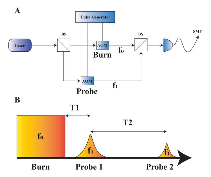
**Figure S1.** (A) Schematic of the setup for generating optical pulses. Laser, Single Frequency MSquared Solistis; BS, Beam Splitter; AOM, Acousto-optic modulator; SMF, Single Mode Fiber;  $f_0$ , Burn frequency;  $f_1$ , Probe frequency. (B) Pulse sequence for time and frequency resolved spectral hole burning. T1 denotes the delay between the Burn and Probe1. T2 denotes the delay between Probe1 and Probe2.
