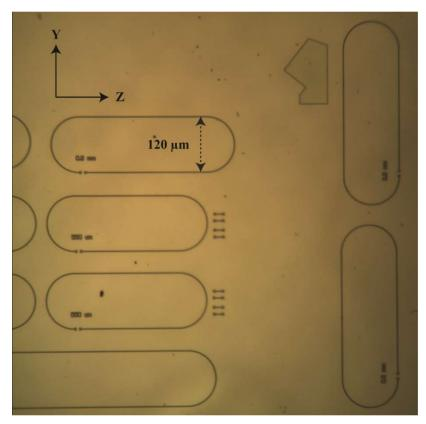
Figure S2. Optical microscope image of a representative sample. The crystal c axis is oriented along the Z direction. Racetrack shaped waveguides are fabricated orthogonally with respect to the c axis of the crystal.
