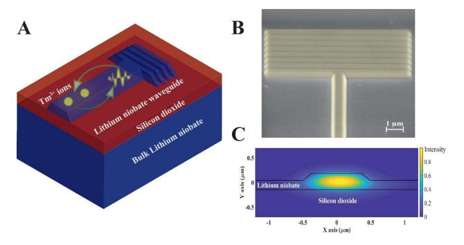
**Figure 1.** (A) Device geometry. Schematic of the cross-section of a waveguide etched in the heterogeneous material stack. (B) Scanning Electron Microscopy image of the waveguide with grating couplers patterned in the Tm<sup>3+</sup> doped lithium niobate thin film. (C) Finite Difference Time Domain simulation showing the electric field distribution along the waveguide cross-section.
