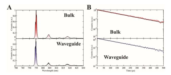
**Figure 3.** (A) Photoluminescence spectrum from bulk crystal and a waveguide in  $\text{Tm}^{3+}$  doped lithium niobate thin film. (B) Time resolved photoluminescence through a thin film waveguide and bulk crystal respectively. The solid black lines denote a fit to a single exponential decay. The fit reveals lifetimes of  $157.4 \pm 1.5 \,\mu\text{s}$  and  $158 \pm 2.8 \,\mu\text{s}$  in the thin film and bulk respectively.
