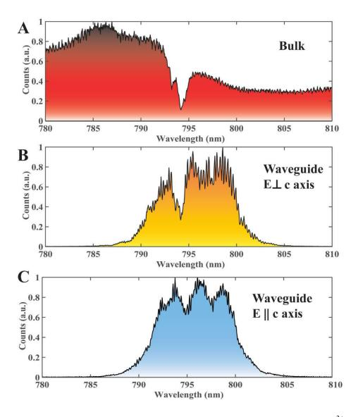
**Figure 2.** (A) Broadband transmission spectrum through a 1 mm length of  $Tm^{3+}$  doped bulk lithium niobate crystal with the electric field polarized perpendicular to the crystal *c* axis. (B)-(C) Broadband transmission spectrum filtered down to 10 nm, through a thin film waveguide with the electric field polarized perpendicular (B) and parallel (C) to the crystal *c* axis.
