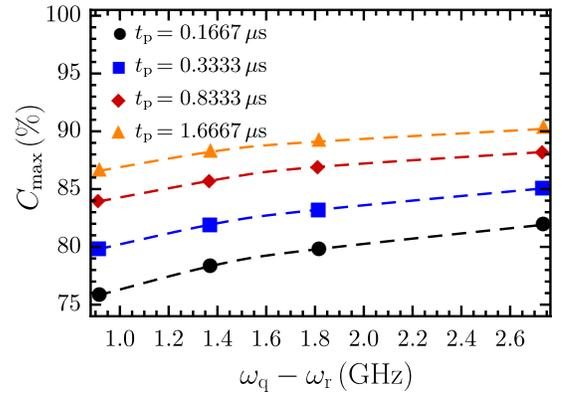
FIG. 6. Dependence of the maximal readout contrast on the detuning between the qubit and resonator for different readout pulse durations  $t_p$ . The rest of the parameters are as described in the caption of Fig. 5.
