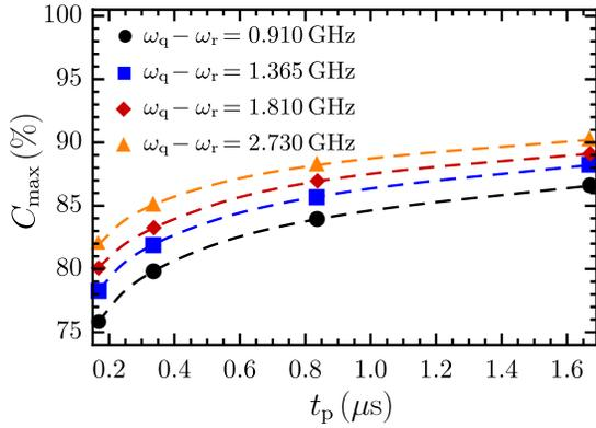
FIG. 5. Dependence of the maximal readout contrast on the readout pulse duration  $t_p$  for different qubit-resonator detunings. To satisfy the criterion (87) we choose  $\lambda/\Lambda = 10$ . The rest of the parameters and notations are the same as in Fig. 4.
