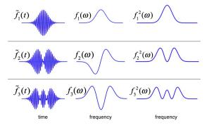
Fig. 5 Examples of a basis set of temporal modes. left: Temporal field, middle: Spectral amplitudes, right: Spectral intensities.
