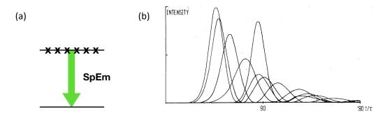
Fig. 1. a) Spontaneous emission from a collection of excited-state atoms evolves into superfluorescence, showing fluctuations (b) in the generated temporal pulse shapes. Fig. (b) reprinted, with permission, from (Haake, *et al* 1979). Copyright (1979) by the American Physical Society.
