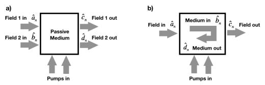
Fig. 6 Nonlinear optical process, with two oscillator systems evolving from initial (input) to final (output) conditions in the presence of laser 'pump' pulses. a) represents optical parametric processes where the medium ends up in the same state in which it began; b) represents a lightmatter coupling that leaves the medium in a state different than where it started.
