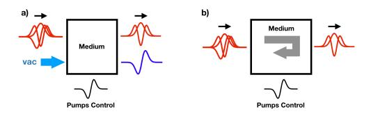
Fig. 8 The Quantum Pulse Gate (QPG). Temporal-mode selectivity and demultiplexing by: a) alloptical frequency conversion, b) medium-based optical memory.
