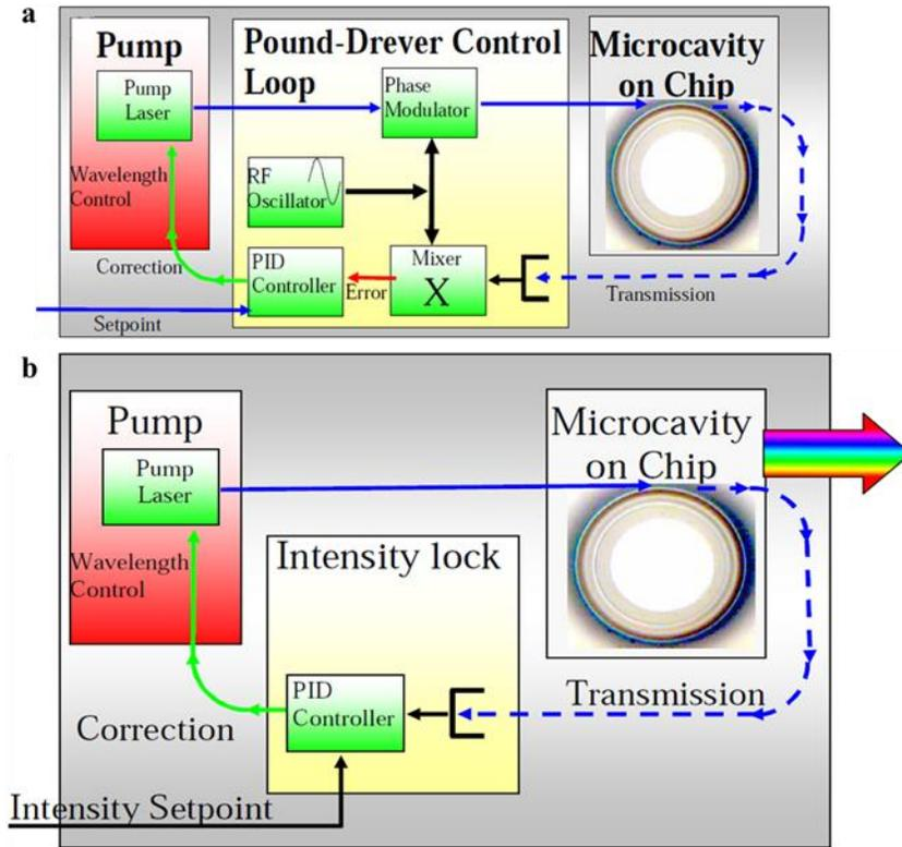
**Fig. 7. Experimental setup of Pound–Drever–Hall (PDH) locking system (a) and thermal locking system (b).**<sup>66</sup> Reprinted with permission from ref.<sup>66</sup> [OSA The Optical Society]
