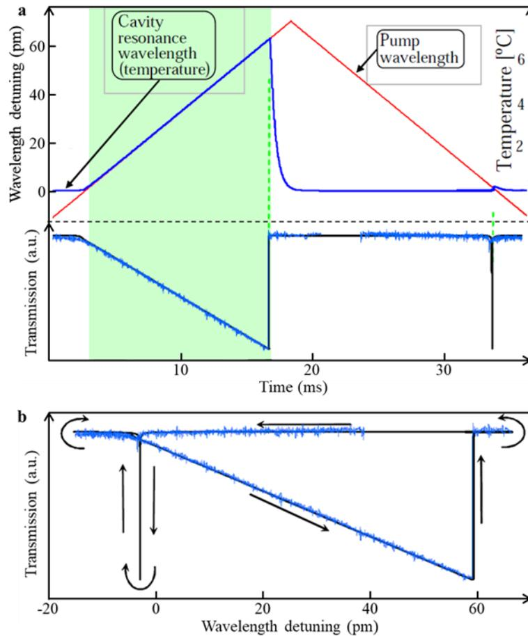
**Fig. 1. Dynamic thermal bistability in a silica microtoroid resonator.**<sup>27</sup> **a** Calculated transmission spectrum, cavity temperature, and resonant wavelength as well as the measured transmission spectrum during the wavelength up- and down-scan processes. **b** Repeating transmission as a function of wavelength detuning in the up-scanning (broadening) and down-scanning (narrowing) processes. Reprinted with permission from ref.<sup>27</sup> [OSA The Optical Society]
