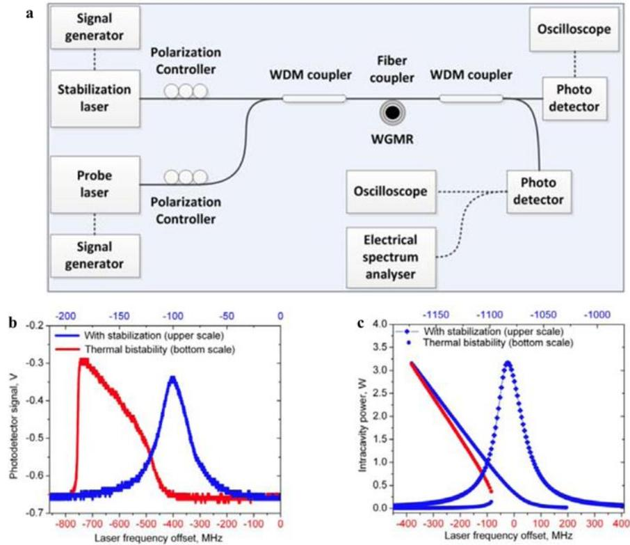
**Fig. 10.** **a** Schematic of the thermal locking stabilization setup. **b** Experimental spectrum of a high  $Q$  WGM with (blue) and without (red) thermal locking stabilization. **c** Simulation results of a high  $Q$  WGM with (blue) and without (red) thermal locking stabilization.<sup>141</sup> Reprinted with permission from ref.<sup>141</sup> [OSA The Optical Society]
