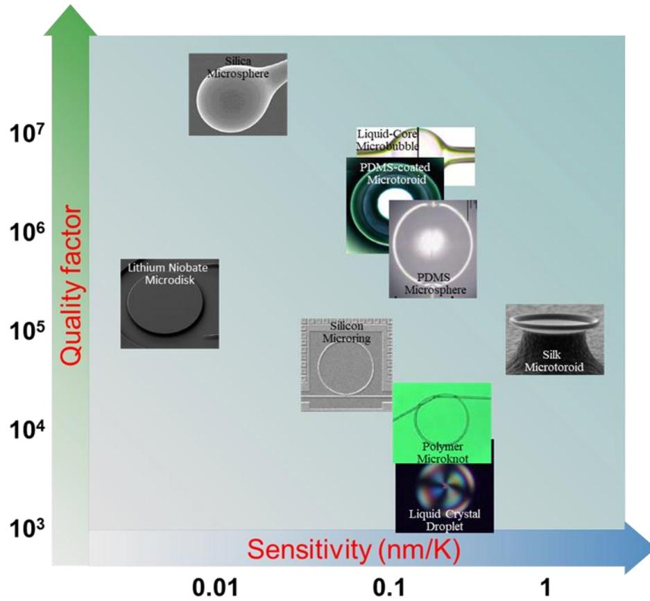
Fig. 6.  $Q$  factor and sensitivity of WGM thermal sensors made of different materials at room temperature.
