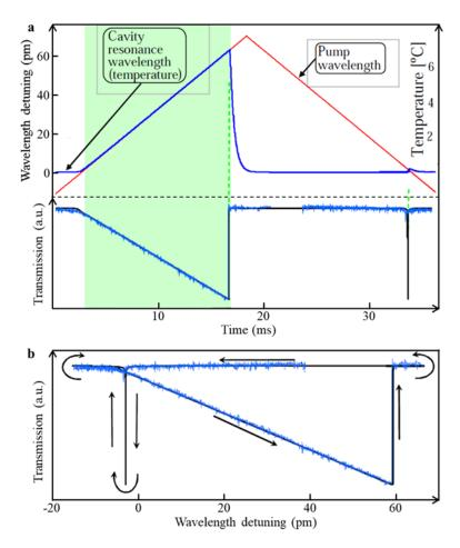
**Fig. 1. Dynamic thermal bistability in a silica microtoroid resonator.**<sup>27</sup> **a** Calculated transmission spectrum, cavity temperature, and resonant wavelength as well as the measured transmission spectrum during the wavelength up- and down-scan processes. **b** Repeating transmission as a function of wavelength detuning in the up-scanning (broadening) and down-scanning (narrowing) processes. Reprinted with permission from ref.<sup>27</sup> [OSA The Optical Society]
