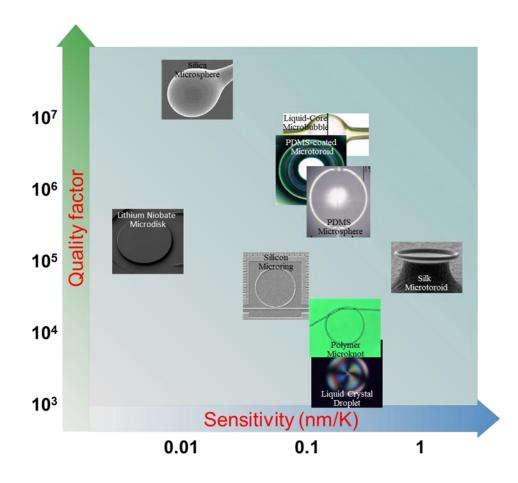
Fig. 6. Q factor and sensitivity of WGM thermal sensors made of different materials at room temperature.
