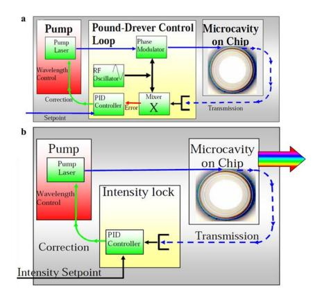
**Fig. 7. Experimental setup of Pound–Drever–Hall (PDH) locking system (a) and thermal locking system (b).**<sup>66</sup> Reprinted with permission from ref.<sup>66</sup> [OSA The Optical Society]
