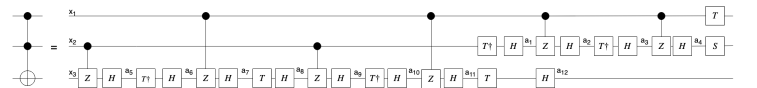
Fig. 8. The polynomial for the Toffoli gate is f_{\mathcal{C}}(x) = x_1 - x_2 - a_2 - a_5 + a_7 - a_9 + a_{11} + 2a_4 + 4(x_1a_6 + x_1a_{10} + x_1a_1 + x_1a_3 + x_2x_3 + x_2a_8 + x_2a_1 + a_1a_2 + a_2a_3 + a_3a_4 + x_3a_5 + a_5a_6 + a_6a_7 + a_7a_8 + a_8a_9 + a_9a_{10} + a_{10}a_{11} + a_{11}a_{12})
