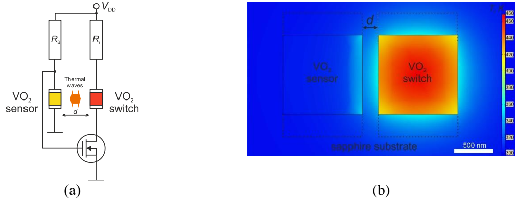
Figure 2. Circuit of the capacitorless model of the oscillator (a), and an example of the temperature distribution on the main switch and sensor at d = 200 nm. The dotted line indicates the region of attachment of the electrodes to the VO 2 film, and the white line indicates the scale.
