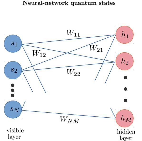
FIG. 2. Schematic depiction of a restricted Boltzmann machine. Every node  $i$  in the visible layer (blue circles) is connected via a weight  $W_{ij}$  with every node  $j$  in the hidden layer (red circles). There are no intra-layer connections. In addition, all nodes are connected to bias nodes (not depicted). For our applications, the number of hidden nodes can always be chosen equal to the number of visible nodes,  $\alpha = N/M = 1$ .
