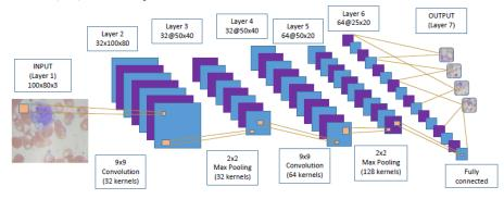
Fig. 2: Architecture of the proposed CNN classifier. The input represents a 2D image, followed by convolution layers and max pooling layers to calculate a set of 32 and then 64 classified feature maps with a fully connected network.
