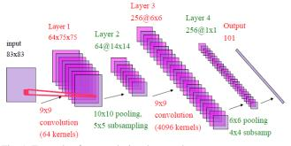
Fig. 1: Example of a convolutional network
