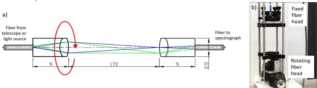
Figure 1. a) Layout and ray trace of the optical double scrambler; b) picture of the rotating scrambler setup.
