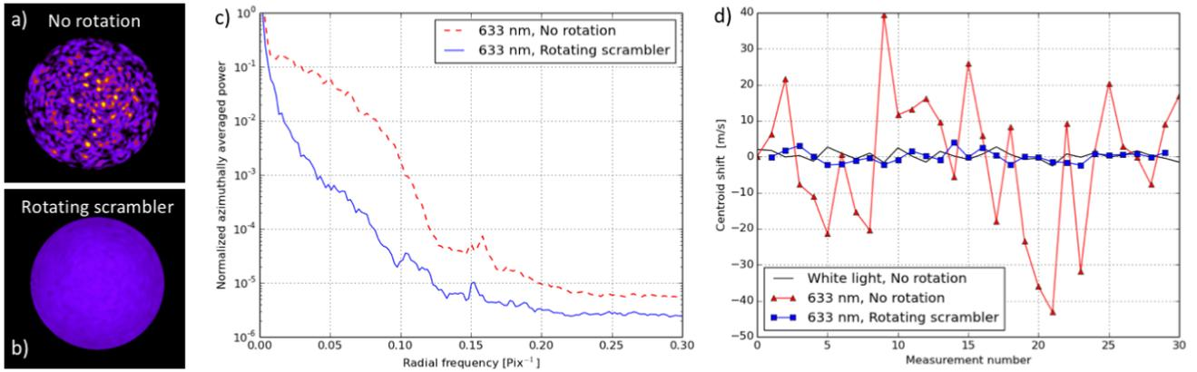
Figure 2. False color images of the fiber exit face a) without and b) with scrambler rotation (same color scale for both images); c) Azimuthally averaged power spectrum of images in a and b; d) Radial velocity scatter of a single spectral line with and without scrambler rotation (white light illumination is shown as noise floor reference).
