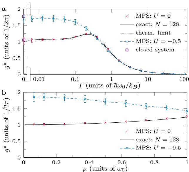
FIG. 4. **Conductance versus temperature and bias.** **a.** Conductance versus the temperature  $T$  at  $\mu = \omega_0/2$ . Closed-system calculations follow Ref. 14 and use  $N = 128$ . **b.** Conductance versus bias  $\mu$  at  $k_B T = \hbar\omega_0/40$ . The setup for the simulations, and the determination of  $I^* = \sigma^* \mu$  and its error, are identical to Fig. 3c.
