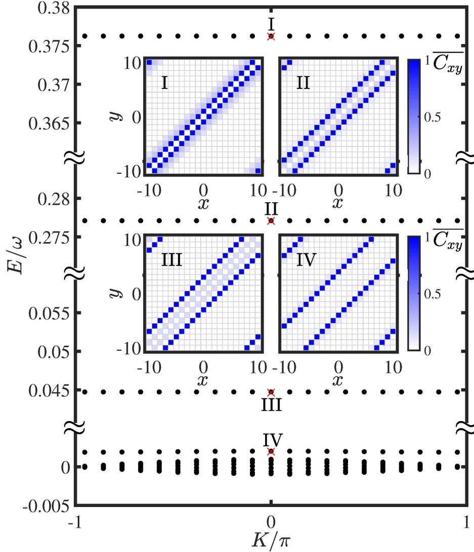
**Figure A2.** (Color online) Quasienergy spectrum  $E$  vs.  $K$ . The insets I, II, III and IV respectively describe the normalized magnon-magnon correlations  $\overline{C_{xy}} = C_{xy}/C_{xy}^{max}$  of Floquet states labeled in the four bound-state band above the continuum band. The parameters are chosen as  $\omega = B = 1$ ,  $\Delta = 0.7$ ,  $J_0 = 1.2$  and  $J_1 = 0.001$ .
