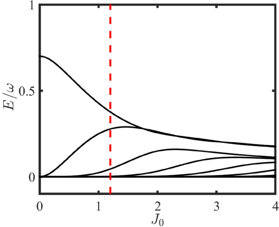
**Figure A1.** (Color online) Quasienergy spectrum  $E$  vs.  $J_0$ . We diagonalize the Floquet-Bloch lattice model (12) with  $\omega = B = 1$ ,  $\Delta = 0.7$  and  $J_1 = 0.001$ . The red dashed line corresponds to  $J_0 = 1.2$ .
