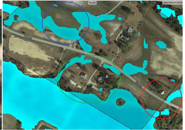
Figure 10: A simulated flood image of Neuse Farms on 19 September 2019, after the hurricane.
