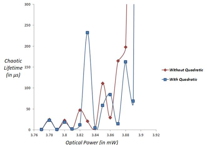
FIG. 7: The chaotic lifetime (in  $\mu s$ ) is shown as a function of the optical power ( $P_o$ ) for linear (red line-diamond) and non-linear case (blue line-square) for relative phase  $\phi = \frac{3\pi}{2}$ . The other parameters are the same as in Fig 2
