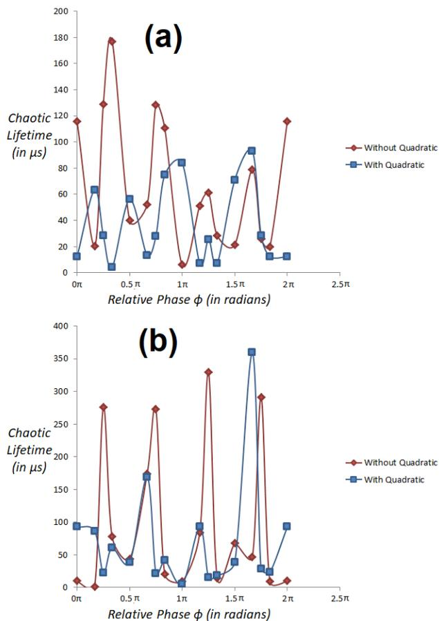
FIG. 5: The chaotic lifetime (in  $\mu s$ ) is shown as a function of the relative phase between optical and microwave fields ( $\phi$ ) for linear (red line-diamond) and non-linear case (blue line-square) at different microwave powers- (a)  $P_a = 28.6 \mu W$ , (b)  $P_a = 45.1 \mu W$ . The other parameters are the same as in Fig 2
