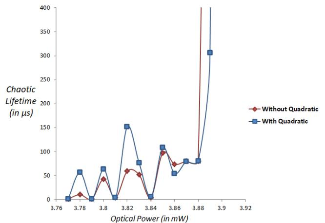
FIG. 6: The chaotic lifetime (in  $\mu s$ ) is shown as a function of the optical power ( $P_o$ ) for linear (red line-diamond) and non-linear case (blue line-square). The other parameters are the same as in Fig 2 with  $\phi = 0$ .
