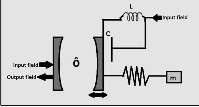
FIG. 1: Schematic of a hybrid Electro-Optomechanical system (EOMS)
