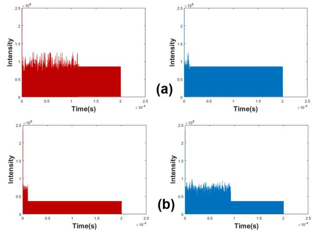
FIG. 4: The intracavity field intensity  $I_o$  vs  $time$  is shown for the linear coupling case (left-red) and non-linear case (right-blue) at different microwave powers- (a)  $P_a = 28.6 \mu W$ , (b)  $P_a = 45.1 \mu W$  over a time interval of  $[0, 200 \mu s]$ . The other parameters are the same as in Fig 2
