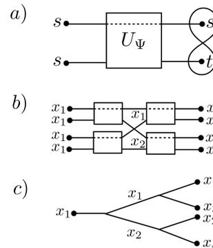
FIG. 3. a) Graphical representation of the map (30), b) example of a circuit for 4 qubits, c) associated branching of qubits into four points of space.
