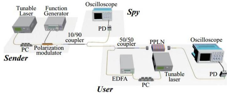
Fig. 3. The experimental setup. The sender, user, and spy are labeled with three shaded squares under the instruments. PC: polarization controller, PD: photoelectric detector, EDFA: erbium-doped fiber amplifier.
