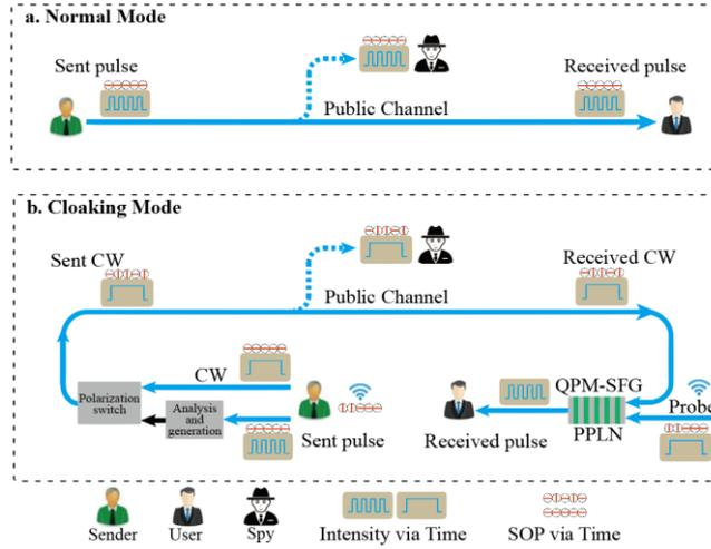
Fig. 1. Schematic of temporal pulse cloaking. a. The sender delivered a pulse to the user in a public channel. b. The pulse delivered in a public channel was cloaked. The blue arrow line denotes optical wave and the black one denotes electric signal. QPM SFG: quasi-phase-matching sum-frequency generation.
