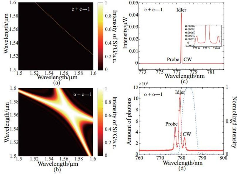
Fig. 2. The simulation (a, b) and experiment (c, d) results for SFG ( $e + e \rightarrow 1$ ) and ( $o + o \rightarrow 1$ )
