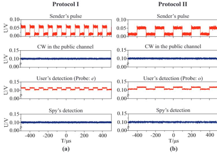
Fig. 4. The result of detection. The cloaking protocols used in the experiment are the protocol I (a) and II (b). For convenience, the CW sent in the public has alternatively  $o$  and  $e$  SOP and the SOP of the probe wave is  $e$  or  $o$  all the time.
