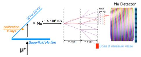
Figure 3. Schema of the MAGE experiment. From Reference 12.
