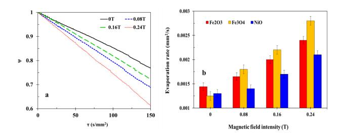
**Figure 3:** (a) Evaporation characteristics of NiO ferrofluids (0.05 wt. %) (b) comparison of evaporation rates of different ferrofluids (0.05 wt. %) as function of magnetic field intensity
