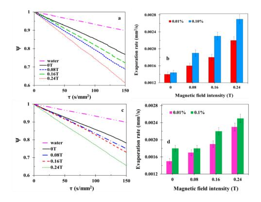
**Figure 2:** (a) Evaporation characteristics of  $Fe_2O_3$  ferrofluids (0.1 wt. %), (b) comparison of evaporation rates of different concentrations (0.01 and 0.1 wt. %) of  $Fe_2O_3$  ferrofluids at different magnetic field intensity, (c) same as (a) but for  $Fe_3O_4$  ferrofluids (0.01 wt. %), (d) same as (b) but for  $Fe_3O_4$  ferrofluids
