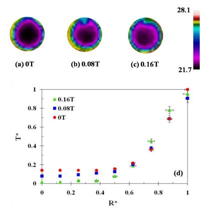
**Figure 6:** Infrared images of the evaporating ferrofluid droplets (0.1 wt. %  $Fe_2O_3$ ) at, (a) 0T, (b) 0.08T, (c) 0.16T, (d) radial distribution of non-dimensional temperature in the droplet. Here
