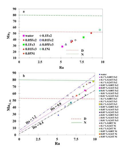
**Figure 8:** (a) Phase plot of the Rayleigh and thermal Marangoni numbers for different ferrofluid droplets evaporating in the absence of magnetic field, (b) comparison of magneto-thermal Marangoni and Rayleigh number for different ferrofluid droplets evaporating in presence magnetic field. 'N' and 'D' lines represent the stability criteria proposed by Nield [38] and Davis [39], respectively.
