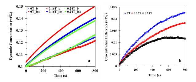
**Figure 9:** (a) The dynamic bulk and interfacial concentration nanoparticles in 0.1 wt. %  $Fe_2O_3$  ferrofluid drop during evaporation under different field strengths, (b) the difference between the two concentrations corresponding to the cases in (a).
