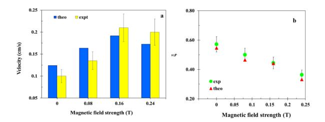
**3.F.** Predicting the ferro-hydrodynamic advection velocity and evaporation rates for the ferrofluid droplets
