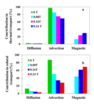
**Figure 7:** (a) Contribution of different mechanisms in the magneto-thermal advection model (0.1 wt. %  $Fe_2O_3$  ferrofluid), (b) contribution of different mechanisms in the magneto-solutal advection model (0.1 wt. %  $Fe_2O_3$  ferrofluid).
