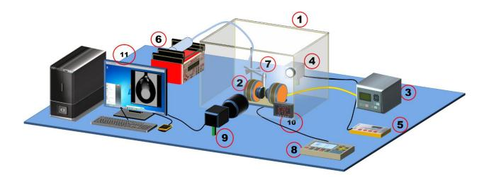
**Figure 1:** Schematic of the experimental setup (1) acrylic chamber, (2) electromagnet with gaussmeter, (3) power supply to electromagnet, (4) LED array for backlight illumination, (5) LED array controller, (6) micro-liter syringe pump, (7) flexible tubing and needle system to generate pendant droplet, (8) gaussmeter control unit, (9) CCD camera with long distance microscope lens, (10) digital thermometer and hygrometer, (11) computer system for camera control and data acquisition.
