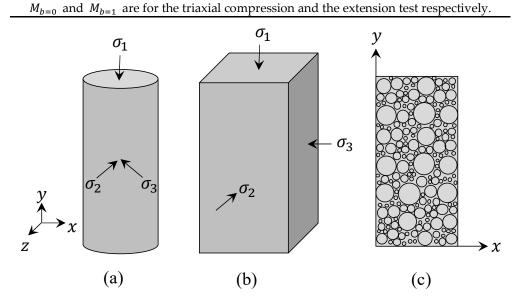
**Figure 4.** The stress condition in triaxial compression/extension tests (**a**) cylindrical sample, (**b**) block sample, (**c**) axisymmetric/biaxial representation of solid and fluids in the sample.
