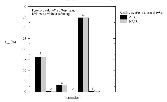
Figure 10. Sensitivity of perturbation for the Kaolin clay.
