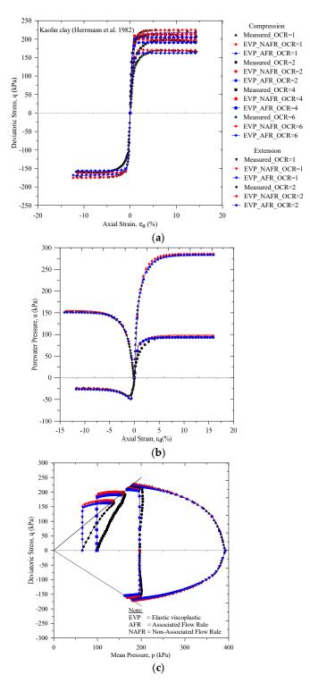
**Figure 7.** Comparison of the measured and the predicted consolidated undrained triaxial compression and the extension tests on the Kaolin clay: (a) the deviatoric stress vs. the axial strain; (b) the porewater pressure vs. the axial strain; and (c) the stress path.
