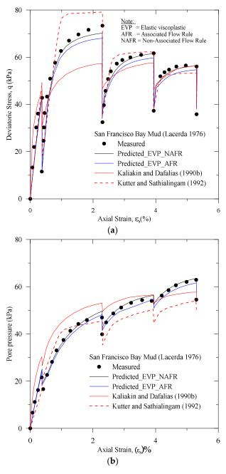
**Figure 6.** Comparison of the measured and the predicted undrained triaxial tests for the stage-changed axial strain rate combined with stress relaxation on the SFBM clay: (a) the deviatoric stress vs. axial strain; and (b) the pore pressure vs. axial strain.
