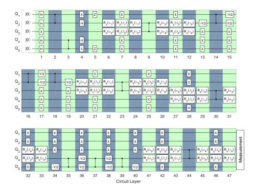
Figure 6: Gate sequences for the test of random unitaries. The initial state of the target qubit is  $|1\rangle$ . The total depth is 47, including 12 double-qubit gates and 119 single-qubit gates.
