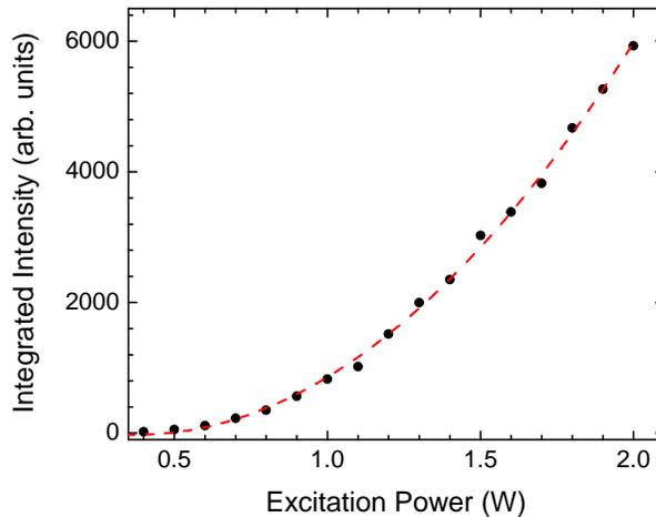
Figure 8: Integrated fluorescence (black circles) of the  $\text{Rb}(6p) \rightarrow \text{Rb}(5s)$  atomic transition following non-resonant excitation by a 780 nm wavelength laser beam, measured for different excitation powers, along with a quadratic fit (red dashed line). The data are taken at a temperature of 673 K for 150 bar argon buffer gas pressure.
