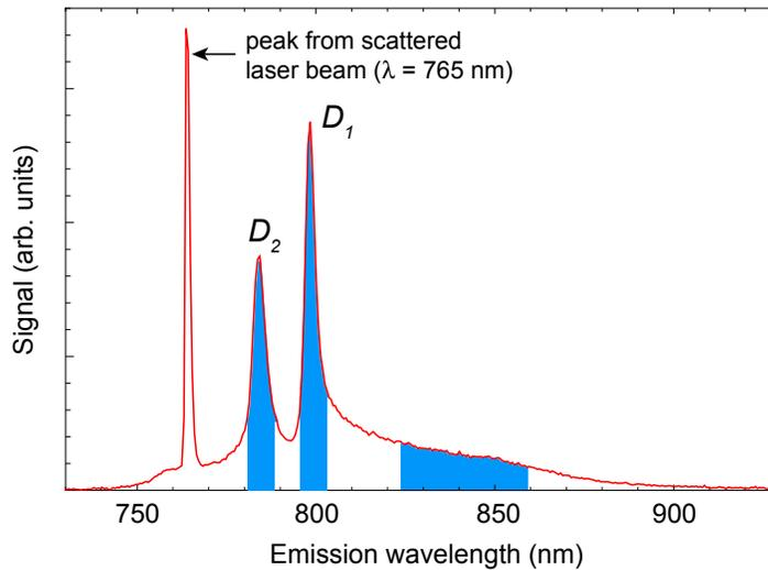
Figure 6: Rubidium fluorescence spectrum (red line) in the vicinity of the atomic  $D$ -lines for excitation wavelength of 765 nm, at 570 K cell temperature and 160 bar argon buffer gas pressure. The integrated area between 824 nm - 860 nm is used to produce the respective fluorescence yield. The areas under the  $D_1$  and  $D_2$  resonances are used for cross-reference.
