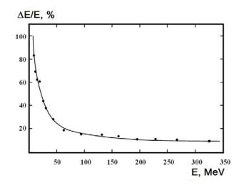
**Fig. 5.** Dependence of the energy resolution  $\Delta E/E$  of TAChS ( $\Delta E$  and *E* being the full width at half maximum of the energy spectrum and the average electron energy, respectively) on the energy of the quasi-monochromatic electron beam (E).
