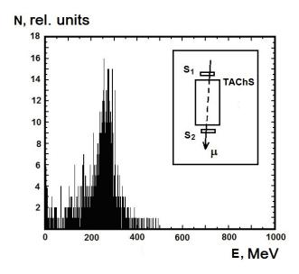
Fig. 2. Calibration spectrum of cosmic muons measured by the TAChS. In the insert:  $S_1$  and  $S_2$  are scintillation counters.
