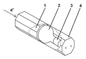
Fig. 1. Scheme of the total absorption Cherenkov spectrometer (TAChS): 1 =radiator, 2 =PMT-49, 3 =voltage divider, 4 =housing.
