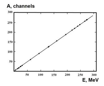
**Fig. 4.** Dependence of the amplitude A of the TAChS signal on the energy *E* of the quasi-monochromatic electron beam.
