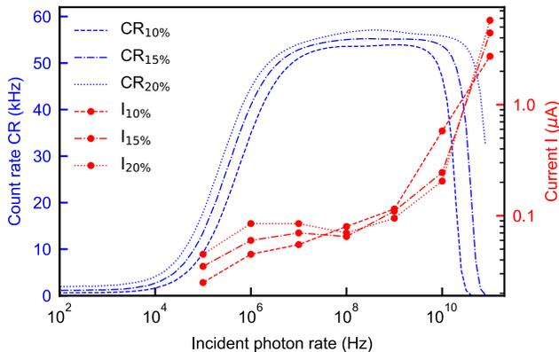
FIG. 7. Dependence of the detector D2 count rate and bias current on the incident photon rate. Unlike measurements done with Si detector in<sup>10</sup>, here we observe a plateau for the count rate due to the deadtime.
