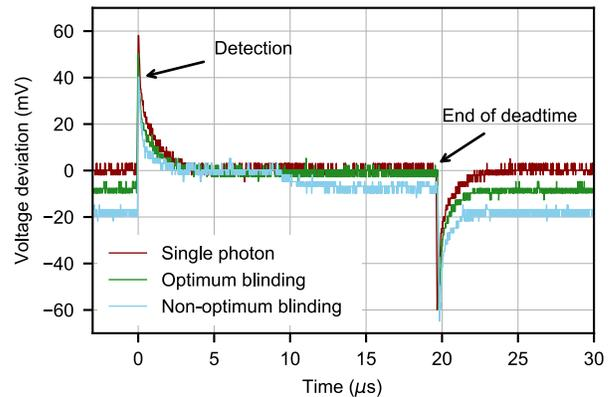
FIG. 8. Fluctuations of the bias voltage due to the detection of a single photon (dark red oscilloscope trace) and under the blinding attack (green and blue oscilloscope traces). For an optimum blinding, we use the minimum blinding power and the blinding laser is switched on just at the end of the deadtime. For non-optimum blinding, the laser is switched on in the middle of the deadtime and has higher power.
