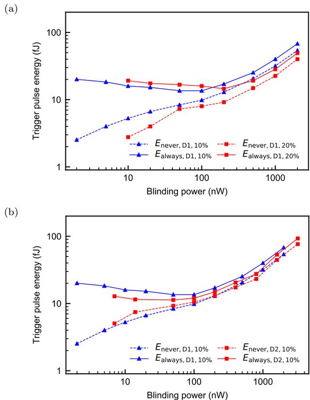
FIG. 4. Dependence of  $E_{always}$  and  $E_{never}$  on the blinding power. (a) Thresholds for detector D1 with 10% and 20% efficiency (corresponding to 1.3 V and 4.1 V excess bias). (b) Comparison of detectors D1 and D2 with the efficiencies set at 10%.
