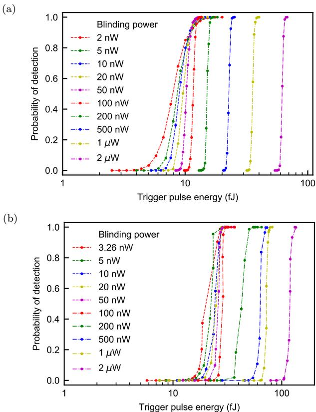
FIG. 3. Probability to force a detection as a function of the pulse energy for (a) detector D1 with 10% photon counting efficiency, and (b) detector D3 with 2 V excess bias above  $V_{br}$ . The measurements were made by sending trigger pulses at a frequency of 40 kHz.
