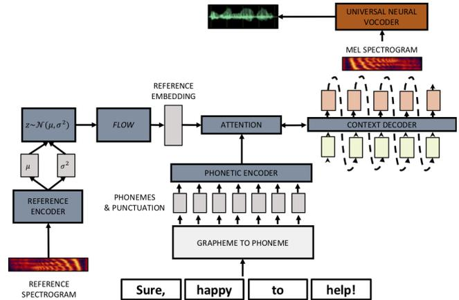
**Fig. 1:** Overview of the system’s architecture: a Variational seq-to-seq auto-encoder conditioned on the phonetic sequence. The Universal Neural Vocoder translates the generated spectrogram into the final speech signal.
