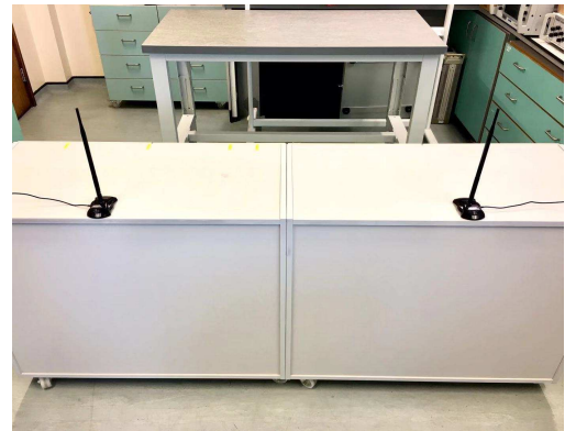
Fig. 8. Receiver side users. N_{user}=2 and each user has N_{RX}=1 antenna.
