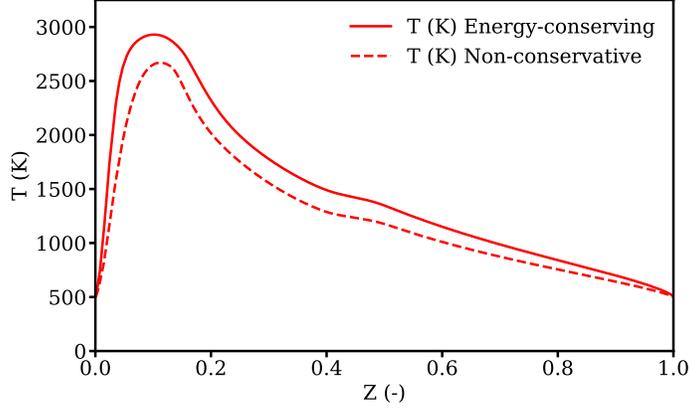
**Figure 10.** Comparison of the temperature profiles obtained with the energy-conserving model (continuous line) and the non-energy-conserving one (dashed line). Same conditions as in Fig. 7 with 0.5 injected  $\text{TiCl}_4$  mass fraction:  $Y_{\text{TiCl}_4}^{\text{inj}} = 0.5$ .
