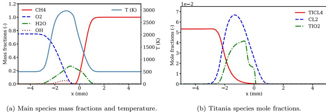
**Figure 7.** Main species profiles for the 1D counterflow  $\text{CH}_4/\text{O}_2$  flame. The inlet temperature is 500 K. Injected  $\text{TiCl}_4$  mass fraction  $Y_{\text{TiCl}_4}^{\text{inj}} = 0.25$  (oxidizer side:  $x = -\infty$ ). Strain rate  $\alpha = 600 \text{ s}^{-1}$ . The stagnation plane is located at  $x = 0$  mm. Results are obtained using the conservative model for mass and enthalpy.
