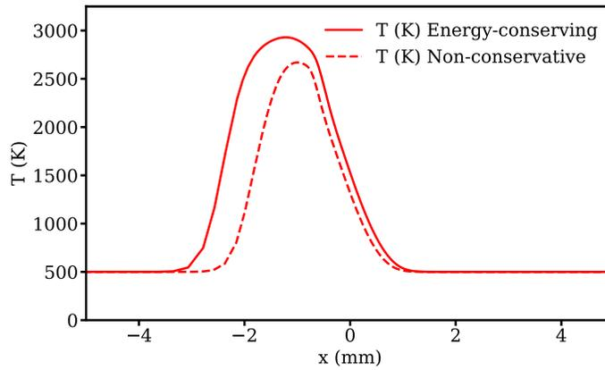
**Figure 9.** Comparison of the temperature profiles obtained with the energy-conserving model (continuous line) and the non-energy-conserving one (dashed line). Same conditions as in Fig. 7 with 0.5 injected  $\text{TiCl}_4$  mass fraction:  $Y_{\text{TiCl}_4}^{\text{inj}} = 0.5$ .
