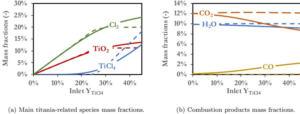
**Figure 6.** Comparison of the burnt gas mass fractions obtained with the energy-conserving model (continuous lines) and the non-energy-conserving one (dashed lines), for varying values of inlet  $\text{TiCl}_4$  mass fraction. The fresh gas composition corresponds to  $\phi = 0.8$ .
