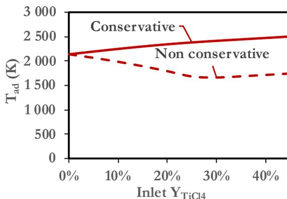
**Figure 5.** Comparison of the burnt gas adiabatic temperatures obtained with the energy-conserving model (continuous line) and the non-energy-conserving one (dashed line), for varying values of inlet TiCl<sub>4</sub> mass fraction. The fresh gas composition corresponds to  $\phi = 0.8$ .
