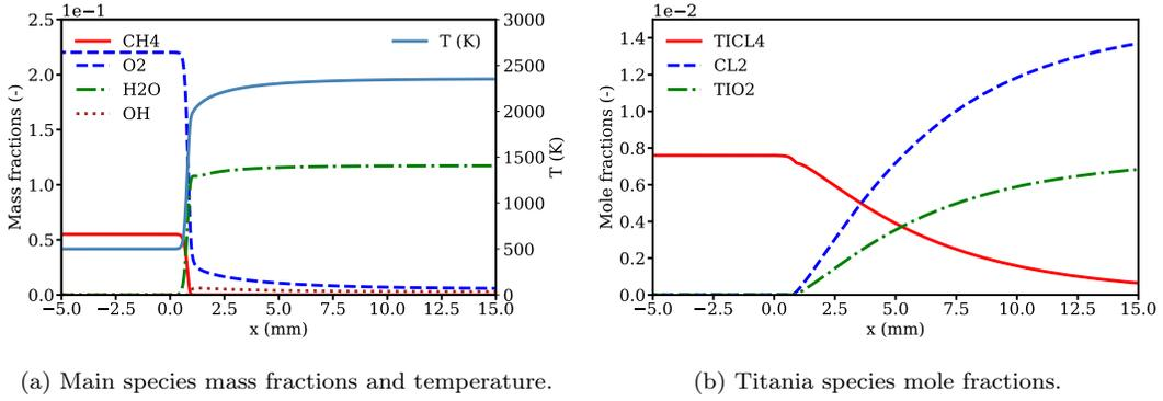
**Figure 2.** Main species and temperature profiles for the 1D premixed  $\text{CH}_4/\text{TiCl}_4/\text{O}_2/\text{N}_2$  flame at stoichiometric conditions. The inlet temperature is 500 K. Injected  $\text{TiCl}_4$  mass fraction  $Y_{\text{TiCl}_4}^{\text{inj}} = 5 \cdot 10^{-2}$ . Results are obtained using the conservative model.
