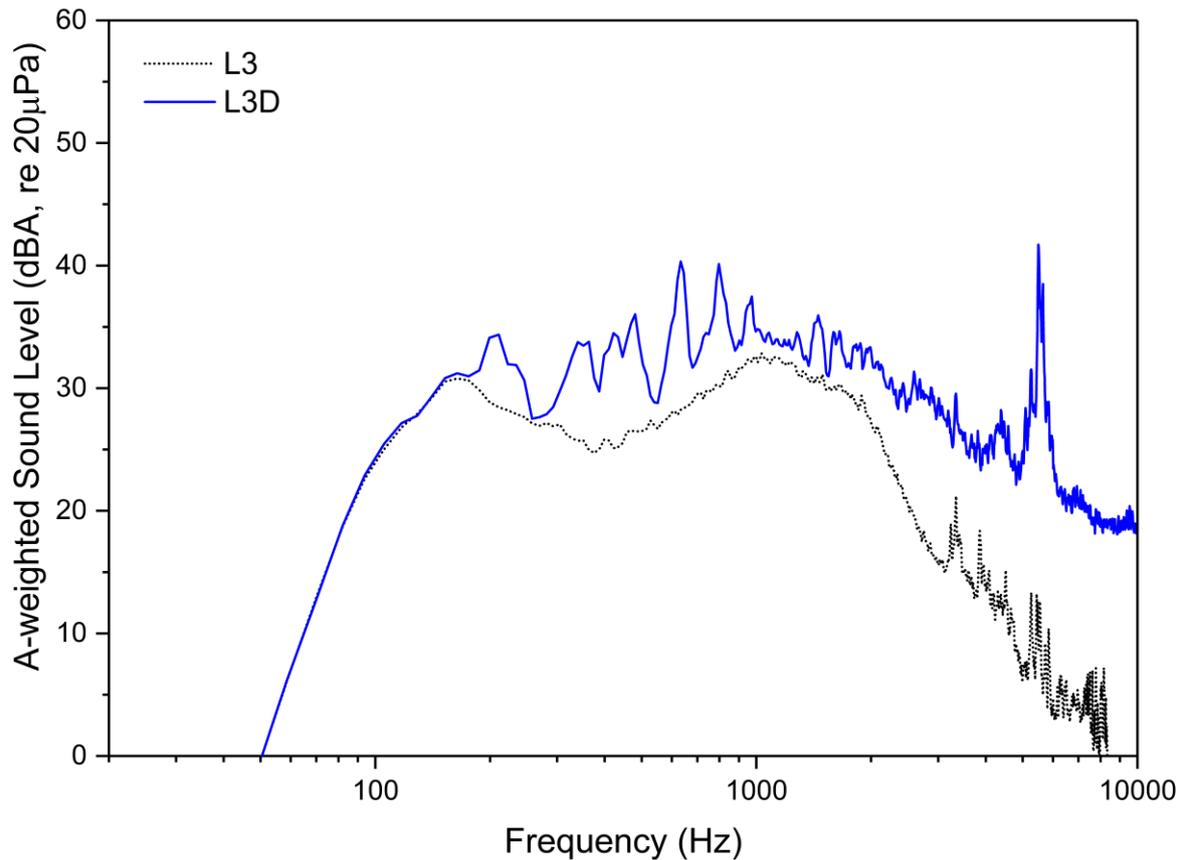
Figure 14. Frequency spectra (A-weighted Sound Pressure Level (dBA, re 20µPa)) measured in locations L1 (top), L2 (middle) and L3 (bottom), without (dotted line) and with (solid line) noise of the small quadcopter.
