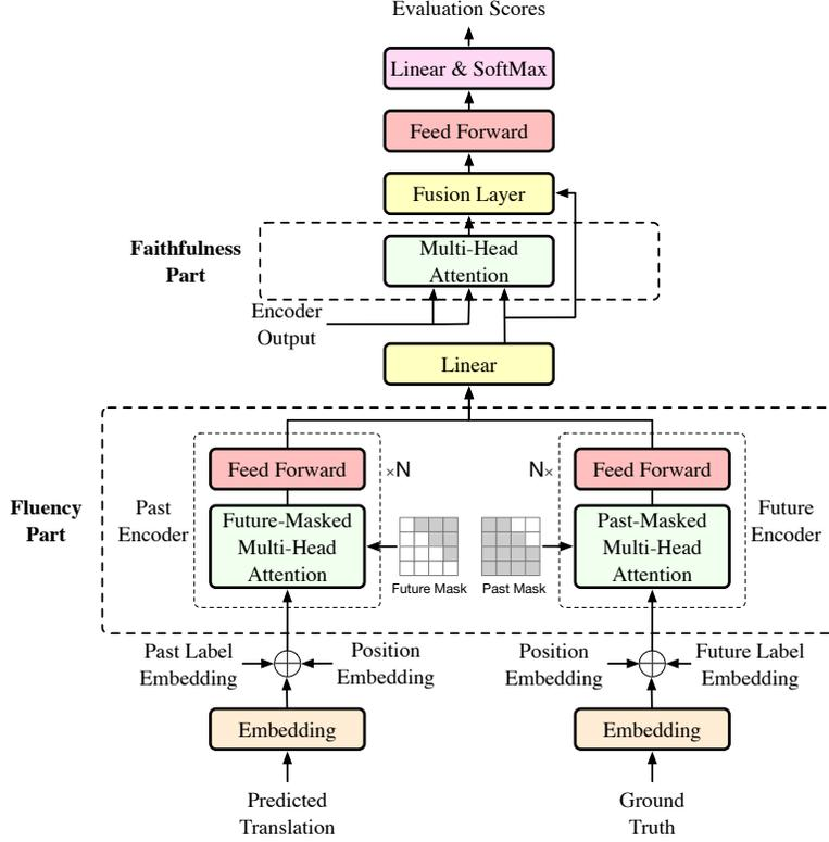
Figure 2: The architecture of the evaluation module.
