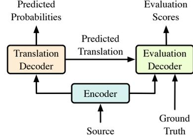
Figure 1: The architecture of the proposed method.
