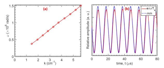
Figure 4: (a) Experimentally obtained dispersion curve ( $\omega$  vs k) for  $\omega_{pi} = 2 \times 10^6$  Hz and  $\lambda_{De} = 0.08$  mm, and (b) Temporal evolution of normalized plasma density, n and potential,  $\phi$  fluctuations.
