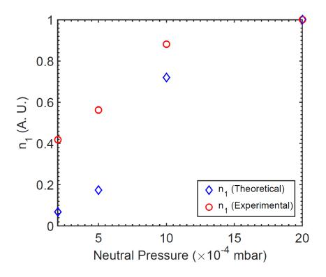
Figure 10: Variation of perturbed density amplitude  $(\mathbf{n_1})$  with neutral pressure, experimental values are shown by circle and theoretically calculated values using Eq(1) are shown by diamond marker.
