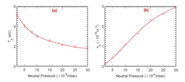
Figure 2: Variation of (a) electron temperature,  $T_e$ , and (b) plasma density,  $\mathbf{n}$  at  $\mathbf{R} = \mathbf{0}$  cm, as a function of neutral pressure for -50 V discharge voltage.
