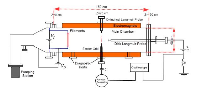
Figure 1: Schematic of the Experimental Device and exciter circuit
