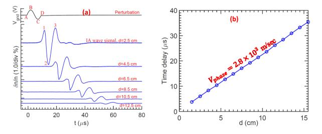
Figure 3: (a) Shows a temporal evolution of density perturbation  $(\delta n/n)$  at different axial locations, and (b) time delay of the first peak of wave as the receiver probe moves away from the exciter grid along the z-axis for - 50 V discharge voltage,  $30 \times 10^{-4}$  mbar neutral pressure, and 100 kHz perturbation frequency, here d is the distance between exciter grid and receiver probe.
