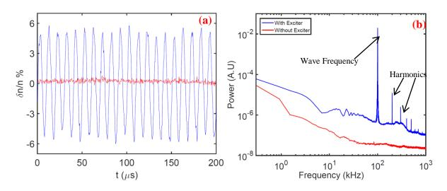
Figure 5: (a) Time evolution of normalized density fluctuation,  $\delta n/n$ , the red trace shows the density fluctuation of quiescent plasma, and blue trace shows the density fluctuation when perturbation of  $2V_{p-p}$  and 100 kHz is excited in plasma. (b) shows the power spectrum of both the signals the lower trace (red) is for quiescent plasma and the upper trace is when the perturbation of  $2V_{p-p}$  and 100 kHz is excited in plasma. The signal is recorded at d=4.5 cm.
