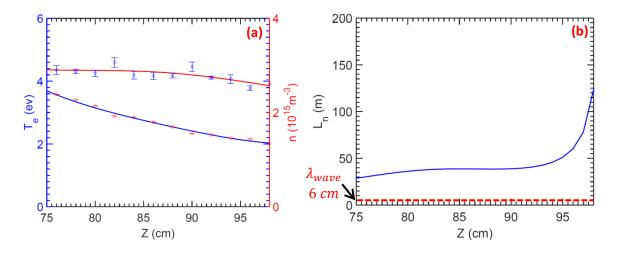
Figure 7: Axial variation of (a) electron temperature,  $T_e$ , and plasma density, n, and (b) plasma density scale length,  $L_n$  the dotted line shows value of IA wavelength ( $\lambda_{wave}$ ) for -50 V discharge voltage and neutral pressure  $5 \times 10^{-4}$  mbar. The exciter grid is placed at Z=75 cm.
