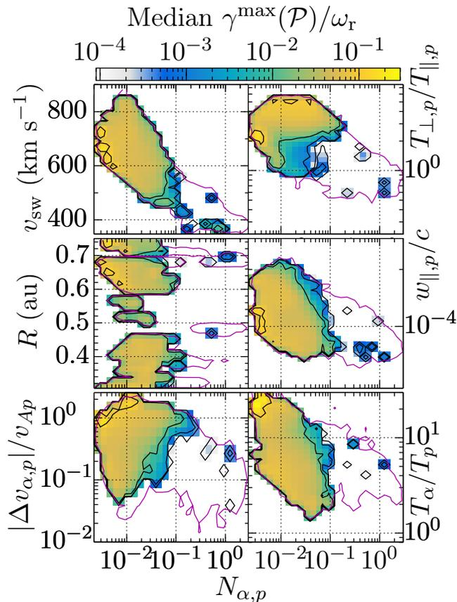
**Figure 6.** Median Growth rate  $\gamma^{\max}/\omega_r(\mathcal{P})$  as a function of Coulomb number  $N_{\alpha,p}$  and solar wind speed  $v_{\text{sw}}$  (top left), radial distance  $R$  (middle left), ion drift speed (bottom left), proton temperature anisotropy  $T_{\perp,p}/T_{\parallel,p}$  (top right), normalized proton thermal speed  $w_{\parallel,p}/c$  (middle right), or ion temperature disequilibrium  $T_{\alpha}/T_p$  (bottom right).
