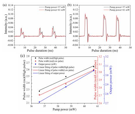
Fig. 7. Tuning the pump power from 57 mW to 61 mW. (a)(b) Oscilloscope trace of pulse evolution under two different states; (c) The pulse width of the first pulse of the low-intensity pulses in the state of three pulses, the pulse width of the first pulse of the high-intensity pulses in the state of three pulses, and average output power in function of pump power.
