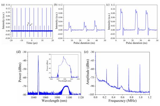
Fig. 6. Period doubling bifurcation of three-pulses DSR. (a) Pulse train; (b)(c) Corresponding to the details of three-pulses DSR under two different states; (d) Corresponding optical spectrum. Inset: local amplification of the corresponding optical spectrum; (e) RF spectrum with a span of 1.2 MHz and a resolution bandwidth of 10 Hz.
