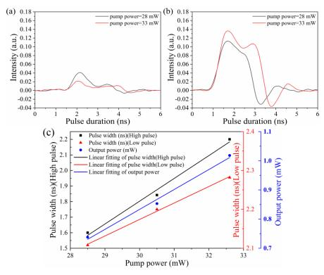
Fig. 3. Tuning the pump power from 28 mW to 33 mW. (a)(b) Oscilloscope trace of pulse evolution under two different states; (c) Pulse width and average output power versus pump power.
