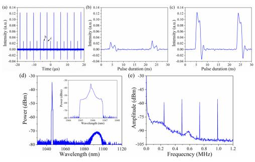
Fig. 4. Period doubling of dual-pulse DSR. (a) Pulse train; (b)(c) Corresponding to the details of dual-pulse DSR under two different states; (d) Corresponding optical spectrum. Inset: zoom-in of the corresponding optical spectrum; (e) RF spectrum with a span of 1.2 MHz and a resolution bandwidth of 10 Hz.
