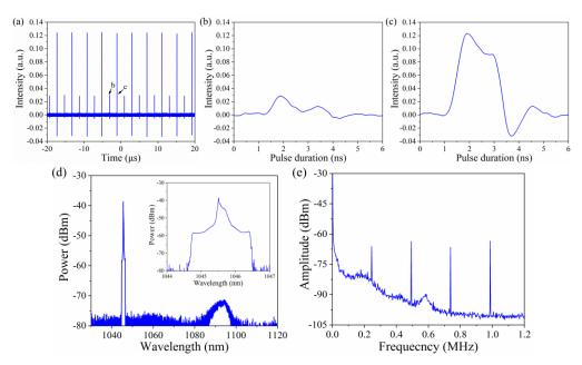
Fig. 2. Period doubling of single DSR pulse. (a) Pulse train; (b)(c) Corresponding to the details of single DSR pulse under two different states; (d) Corresponding optical spectrum. Inset: local amplification of the corresponding optical spectrum; (e) RF spectrum with a span of 1.2 MHz and a resolution bandwidth of 10 Hz.
