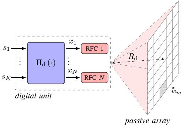
Fig. 1: Block diagram of the RA/TA HAD transceiver.
