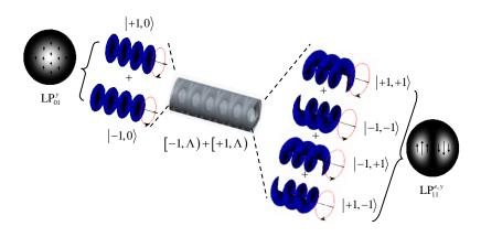
Fig. 6. The sketch of mode conversion in FMF from  $_{LP_{01}^{r}}$  to  $_{LP_{11}^{r,v}}$  by SHGs  $[-1,\Lambda)+[+1,\Lambda)$  with  $\Lambda = 625.0 \ \mu m$ .
