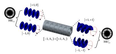
Fig. 3. The sketch of mode conversion from the fundamental modes  $_{HE_{11}}$  to vector modes  $_{HE_{21}}$  by SHGs  $_{[-1,\Lambda_1)+[+1,\Lambda_1)}$  with  $_{\Lambda_1 = 807.4} \mu m$  in RCF.
