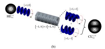
Fig. 5. The sketch of mode conversion in FMF from the left-handed circularly polarized fundamental modes  $_{\text{HE}_{11}}$  to modes  $_{\text{CL}_{11}^{e+1}}$  by SHGs  $_{[-1,\Lambda)+[+1,\Lambda)}$  with  $\Lambda = 625.0 \,\mu\text{m}$  and  $_{\Delta\varphi=0}$  (a), and modes  $_{\text{CL}_{11}^{e+1}}$  by SHGs  $_{[-1,\Lambda)+i[+1,\Lambda)}$  with  $\Lambda = 625.0 \,\mu\text{m}$  and  $_{\Delta\varphi=\pi/2}$  (b).
