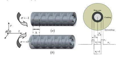
Fig. 2. The diagram of SHGs  $[-1, \Lambda) + \exp(i\Delta\varphi) \cdot [+1, \Lambda)$  formed in the ring core of RCF, (a),  $\Delta\varphi = 0$  and (b),  $\Delta\varphi = \pi/2$ . (c) Cross-section and refractive index distribution of of RCF.
