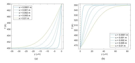
Figure 4: Streamwise evolution of the temperature distributions in the transverse direction for the oxygen/n-decane mixture at p = 150 bar. The interface is located at  $y = 0 \ \mu$ m. (a) liquid temperature; (b) gas temperature.
