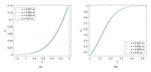
Figure 10: Evolution of the non-dimensional temperature distributions in the transverse direction against the non-dimensional similarity variable,  $\eta^*$ , for the oxygen/n-decane mixture at p = 150 bar. (a) liquid temperature; (b) gas temperature.
