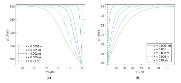
Figure 5: Streamwise evolution of the viscosity distributions in the transverse direction for the oxygen/*n*-decane mixture at p = 150 bar. The interface is located at  $y = 0 \mu m$ . (a) liquid viscosity; (b) gas viscosity.
