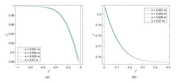
Figure 11: Evolution of the non-dimensional temperature and density distributions in the transverse direction against the nondimensional similarity variable,  $\eta^*$ , for the oxygen/n-decane mixture at p = 150 bar. (a) liquid density; (b) gas density.
