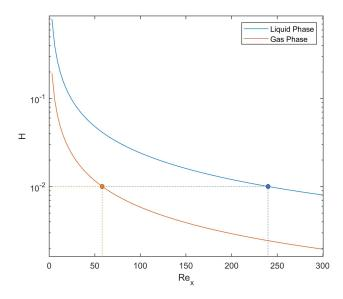
Figure 16: *H* for varying streamwise Reynolds numbers at p = 150 bar.
