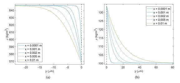
Figure 3: Streamwise evolution of the density distributions in the transverse direction for the oxygen/*n*-decane mixture at p = 150 bar. The interface is located at  $y = 0 \ \mu$ m. (a) liquid density; (b) gas density.
