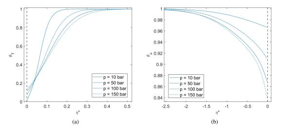
Figure 14: Comparison of the non-dimensional temperature and streamwise velocity distributions in the transverse direction against the similarity variable,  $\eta^*$ , for the oxygen/n-decane mixture at p = 10, 50, 100, and 150 bar and streamwise position x = 1 cm. (a) normalized temperature in the gas phase near the interface; (b) normalized streamwise velocity in the liquid phase near the interface.
