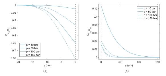
Figure 9: Comparison of the transverse velocity and mole fraction distributions in the transverse direction for the oxygen/n-decane mixture at p = 10, 50, 100, and 150 bar and streamwise distance 1 cm ( $Re_x = 10,000$ ). (a) *n*-decane mole fraction in the liquid phase; (b) *n*-decane mole fraction in the gas phase.
