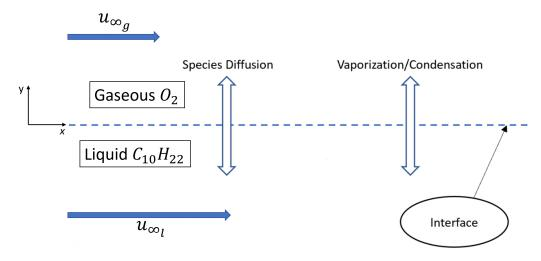
Figure 1: 2D schematic of the mixing layer problem.
