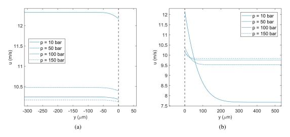
Figure 7: Comparison of the streamwise velocity distributions in the transverse direction for the oxygen/n-decane mixture at p = 10, 50, 100, and 150 bar and streamwise distance 1 cm ( $Re_x = 10,000$ ). (a) liquid streamwise velocity; (b) gas streamwise velocity.
