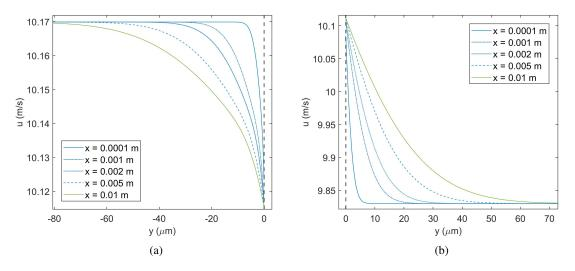
Figure 6: Streamwise evolution of the streamwise velocity distributions in the transverse direction for the oxygen/*n*-decane mixture at p = 150 bar. The interface is located at  $y = 0 \ \mu m$ . (a) liquid streamwise velocity; (b) gas streamwise velocity.
