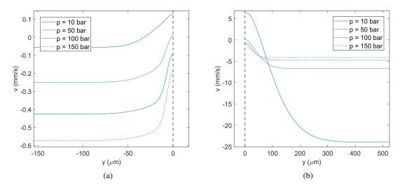
Figure 8: Comparison of the transverse velocity distributions in the transverse direction for the oxygen/n-decane mixture at p = 10, 50, 100, and 150 bar and streamwise distance 1 cm ( $Re_x = 10,000$ ). (a) liquid transverse velocity; (b) gas transverse velocity.
