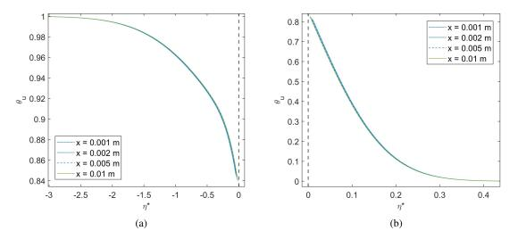
Figure 12: Evolution of the non-dimensional streamwise velocity distribution in the transverse direction against the non-dimensional similarity variable,  $\eta^*$ , for the oxygen/n-decane mixture at p = 150 bar. (a) streamwise velocity in the liquid phase near the interface; (b) streamwise velocity in the gas phase near the interface.
