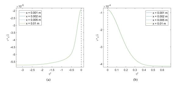
Figure 13: Evolution of the streamwise distance-weighted transverse velocity distribution in the transverse direction against the nondimensional similarity variable,  $\eta^*$ , for the oxygen/n-decane mixture at p = 150 bar. (a) weighted transverse velocity in the liquid phase near the interface; (b) weighted transverse velocity in the gas phase near the interface.
