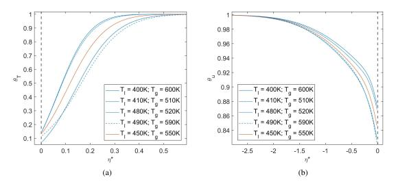
Figure 15: Comparison of the temperature and streamwise velocity distributions in the transverse direction against the similarity variable,  $\eta$  for the oxygen/n-decane mixture at p = 150 bar and streamwise position x = 1 cm. (a) normalized temperature in the liquid phase near the interface; (b) normalized streamwise velocity in the liquid phase near the interface.
