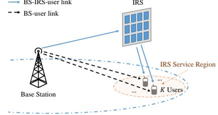
Fig. 1. An IRS-enhanced OFDMA downlink communication system.
