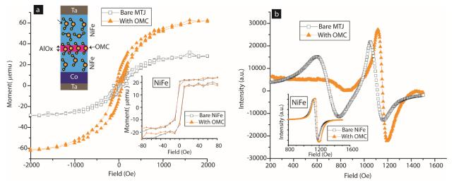
Fig. 4 Magnetic studies of 7000 MTJMSD by SQUID and FMR. (a) SQUID magnetometer study of MTJ before and after hosting OMC channels across AlOx insulator. Top left inset shows that OMC can bridge across AlOx and also bond with the exposed magnetic layers, mainly NiFe. Bottom right inset show magnetic study of NiFe before and after interacting with OMCs. (b) FMR study of MTJ before and after hosting OMC channels. Inset graph shows the impact of OMC on NiFe film only.
