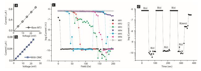
Fig. 2: Current-voltage study of the MTJ (a) before and after attaching (b) OMCs across the tunnel barrier along the exposed edges. (c) Magneto-resistance (MR) studies on MTJMSD showing several orders of change current at 50 mV bias and under in-plane magnetic field. (d) Effect of changing magnetic field direction from inplane to out of the plane on MTJMSD.
