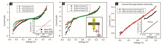
Fig. 3 (a) Stabilized pA level current state on MTJMSD. Inset of this panel shows bare tunnel junction current before and after hosting OMC molecular channels. (b) Effect of changing biasing lead on pA level current state. (c) Current-voltage study through bottom electrode before and after the stabilization of pA level current state.
