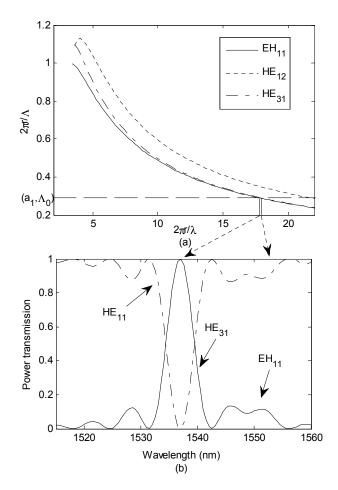
Fig. 6(a) Curves of  $2\pi r/\Lambda$  versus  $2\pi r/\lambda$  for OAMM HE<sub>31</sub>, EH<sub>11</sub>, and HE<sub>12</sub> coupled from HE<sub>11</sub> in a high-index core fiber. (b) Power exchange spectrum from HE<sub>11</sub> to OAMM HE<sub>31</sub>.
