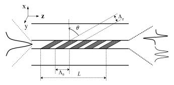
Fig. 3 Structure diagram of tilted optical gratings in a high-NA fiber, and the coupling process from the fundamental mode  $HE_{11}$  (left) to vector modes  $TM_{01}$ ,  $TE_{01}$ ,  $HE_{21}$  or  $HE_{31}$  (right).
