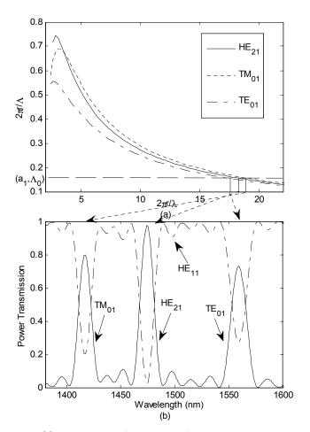
Fig. 5 (a) Curves of  $2\pi r/\Lambda$  versus  $2\pi r/\lambda$  for CSMs and OAMM HE<sub>21</sub> coupled from HE<sub>11</sub> in a naked-core fiber. (b) Power exchange spectrum from HE<sub>11</sub> to these three modes.
