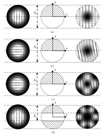
Fig. 4 Relationships between transverse modulation period  $\Lambda_x$  and mode coupling from  $HE_{11}$  to  $TM_{01}$  (a), to  $TE_{01}$  (b), to  $HE_{21}$  (c), and to  $HE_{31}$  (d).
