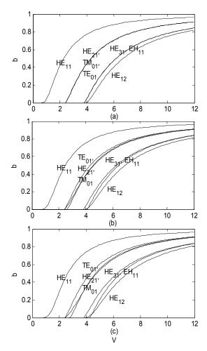
Fig. 1 Modal dispersion curves of several vector modes, (a) ordinary SMF,  $n_1 = 1.4681$ ,  $n_2 = 1.4628$ ; (b) high-index-core fiber  $n_1 = 1.85$ ,  $n_2 = 1.46$ ; (c) naked-core fiber,  $n_1 = 1.4681$ ,  $n_2 = 1.00$ .
