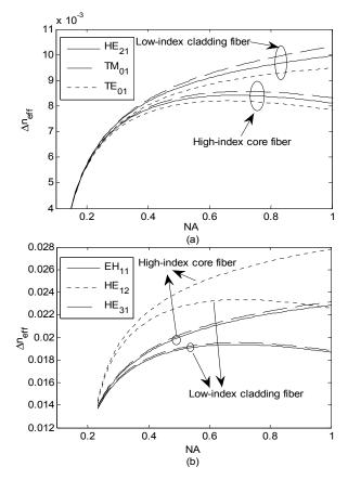
Fig. 2 Relationships between different  $\Delta n_{eff}$  under various *NA* for HE<sub>21</sub>, TM<sub>01</sub>, TE<sub>01</sub> (a), and HE<sub>31</sub>, EH<sub>11</sub>, and HE<sub>12</sub> (b) in both high-index core and low-index cladding fiber.
